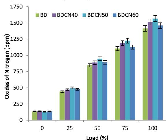
Figure 10. Oxides of Nitrogen Vs Load
