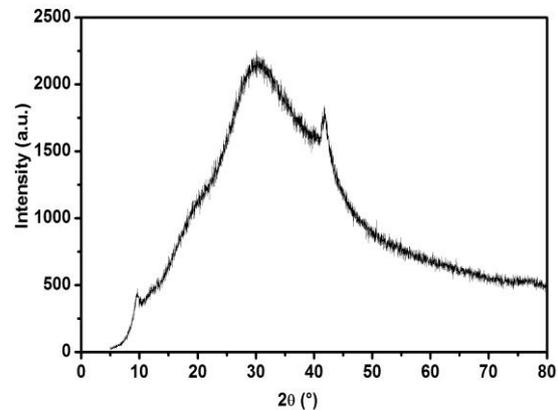
**Figure 5.** X-ray diffraction image of the CNT (Zahra et al. 2017)
