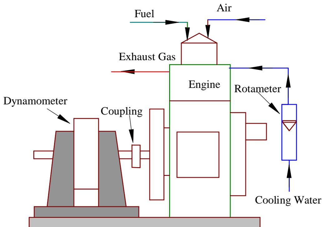
**Figure 4.** Schematic of the engine experimental setup**Table 4.** Comparison of fuel properties
