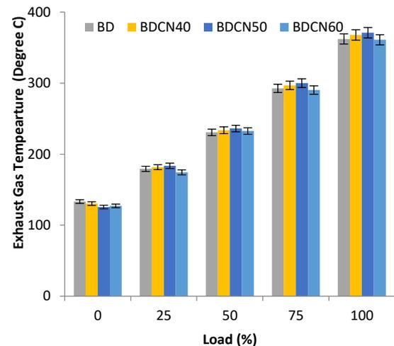
Figure 7. Exhaust Gas Temperature Vs Load
