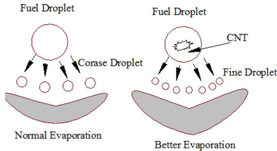
Figure 5. Schematic of fuel droplet breaking and evaporation
