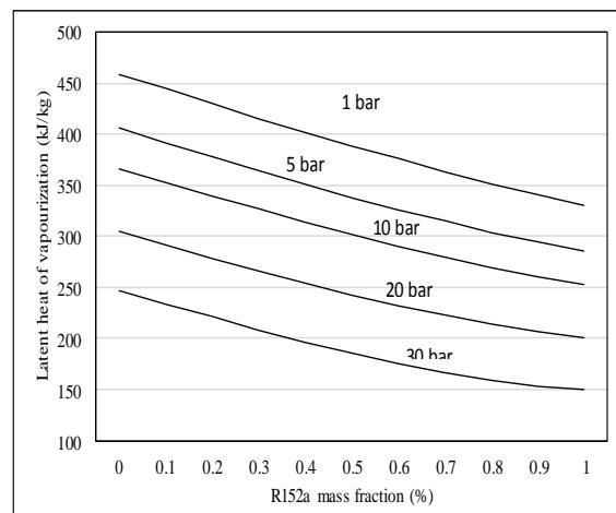
**Figure 2.** Latent heat of vaporization depending on the pressure and R-152a mass fraction
