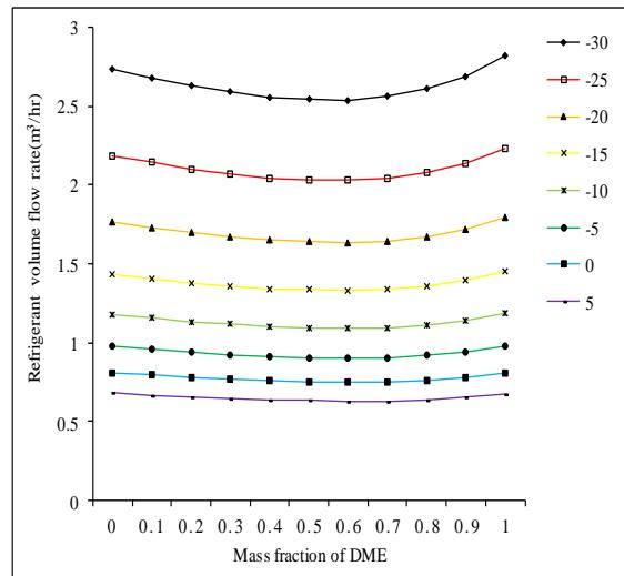
**Figure 10.** Variation of a refrigerant volume flow rate depending on evaporation temperature and DME mass fraction
