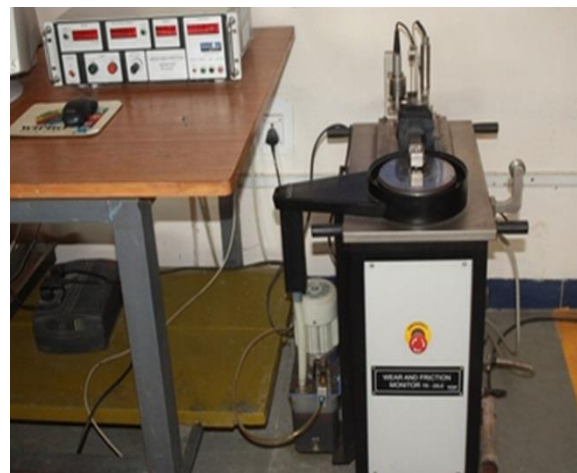
Figure 1. Dry sliding wear test arrangement
