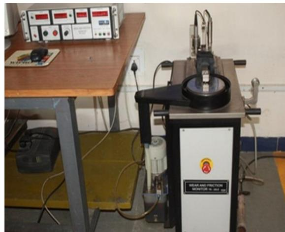
**Figure 1.** Dry sliding wear test arrangement
