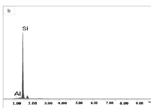
**Figure 2.** (a) SEM image of Al-12Si alloy (b) EDX of Si needle (marked 'A')
