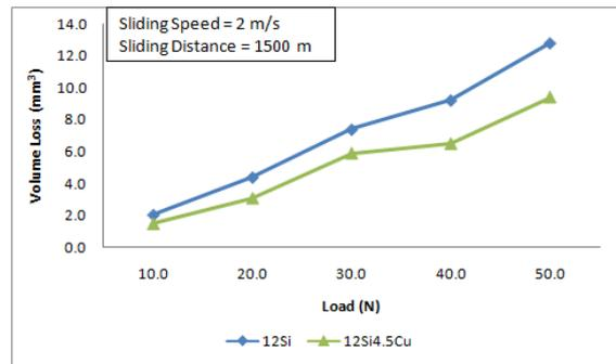
**Figure 4.** Variation of Volume loss with different loads
