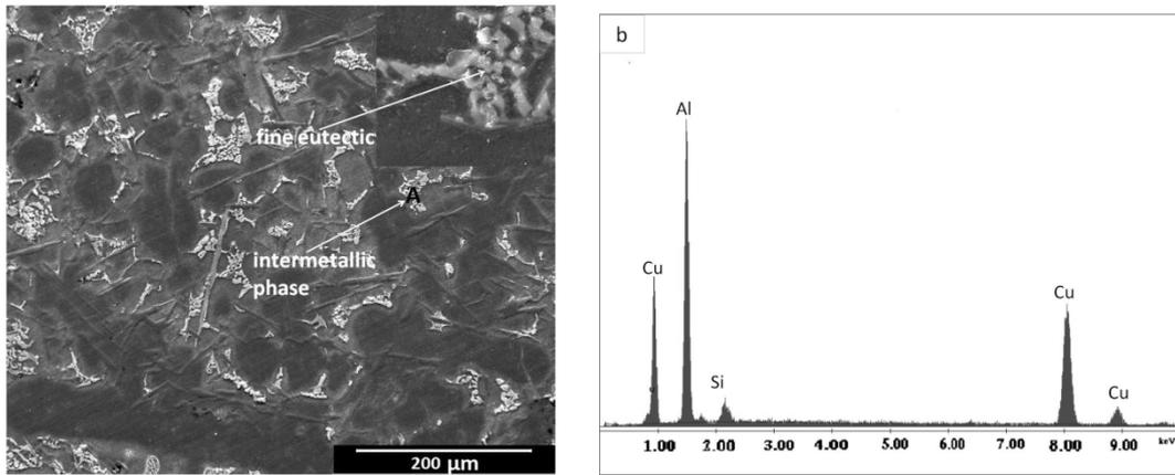
**Figure 3.** (a) SEM image of Al-12Si-4.5Cu alloy (b) EDX of CuAl<sub>2</sub> (marked 'A')
