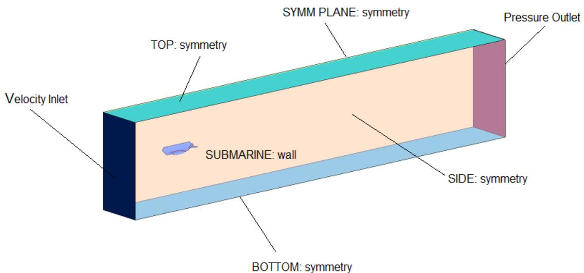
**Figure 7.** Applied boundary conditions on computational domain
