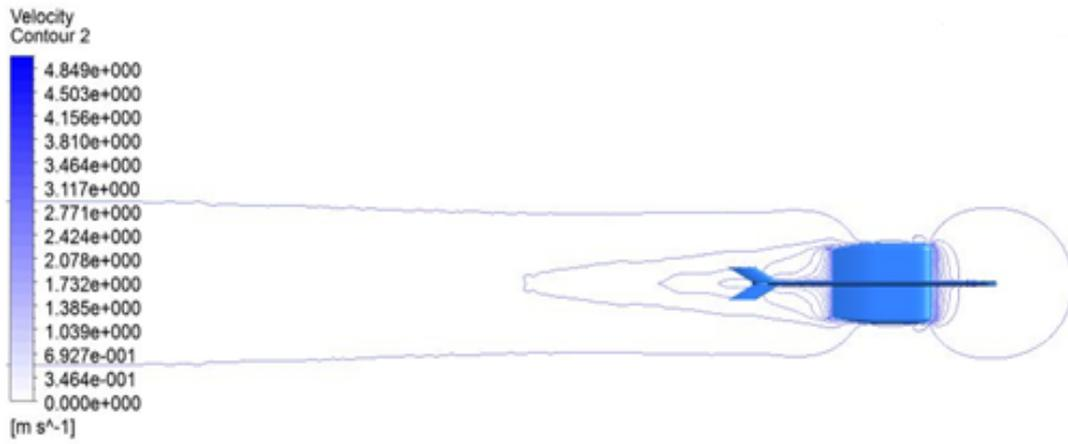
Figure 12. Velocity contours in longitude plane (top view) with zero hydrofoil and 50° tail sweep angle
