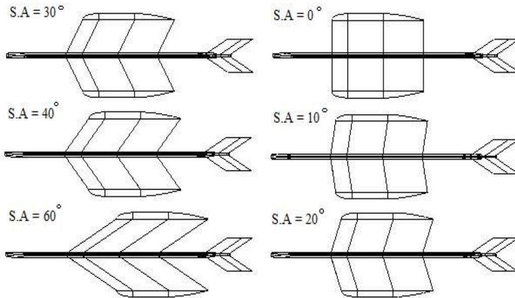
**Figure 4.** Submarine with fixed horizontal tail and swept hydrofoil that change from 0° to 60°
