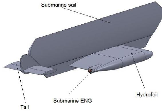
**Figure 1.** Components of studying submarine in basic shape (zero hydrofoil and horizontal tail sweep angle)
