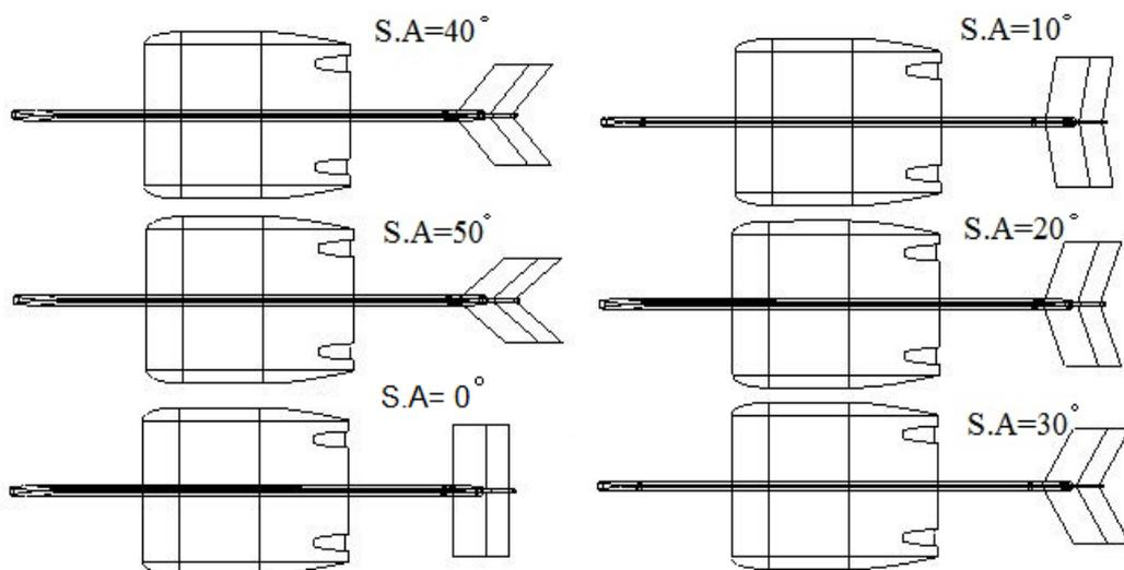
**Figure 3.** Submarine with fixed hydrofoil and swept horizontal tail that change from 0° to 50°
