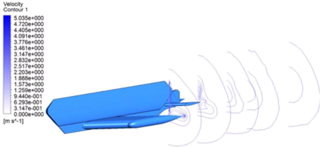
Figure 11. Velocity contours in parallel section planes with 60° hydrofoil and 50° tail sweep angle
