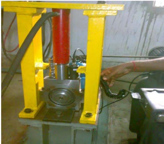
Figure 3. Test bearing with Probes
