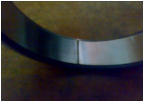
**Figure 5.** Outer race seeded defect (0.5mm width)
