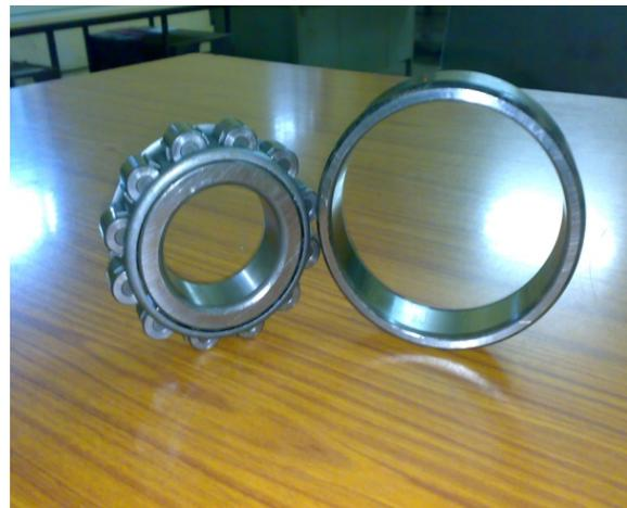
Figure 4. N312 cylindrical roller bearing
