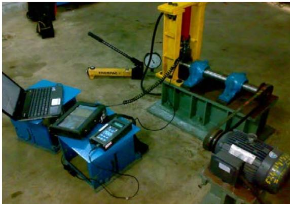
Figure 2. Bearing Test Rig
