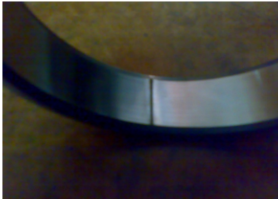
Figure 5. Outer race seeded defect (0.5mm width)
