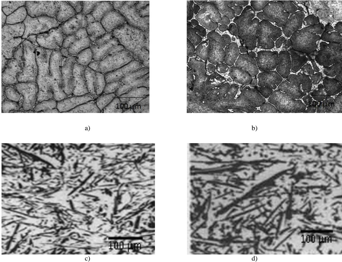
**Figure 2.** The microstructure of Al/ basalt short fiber composites containing a) 0 wt.%, b) 2.5 wt.%, c) 7.5 wt.%, d) 10 wt.% basalt short fiber.
