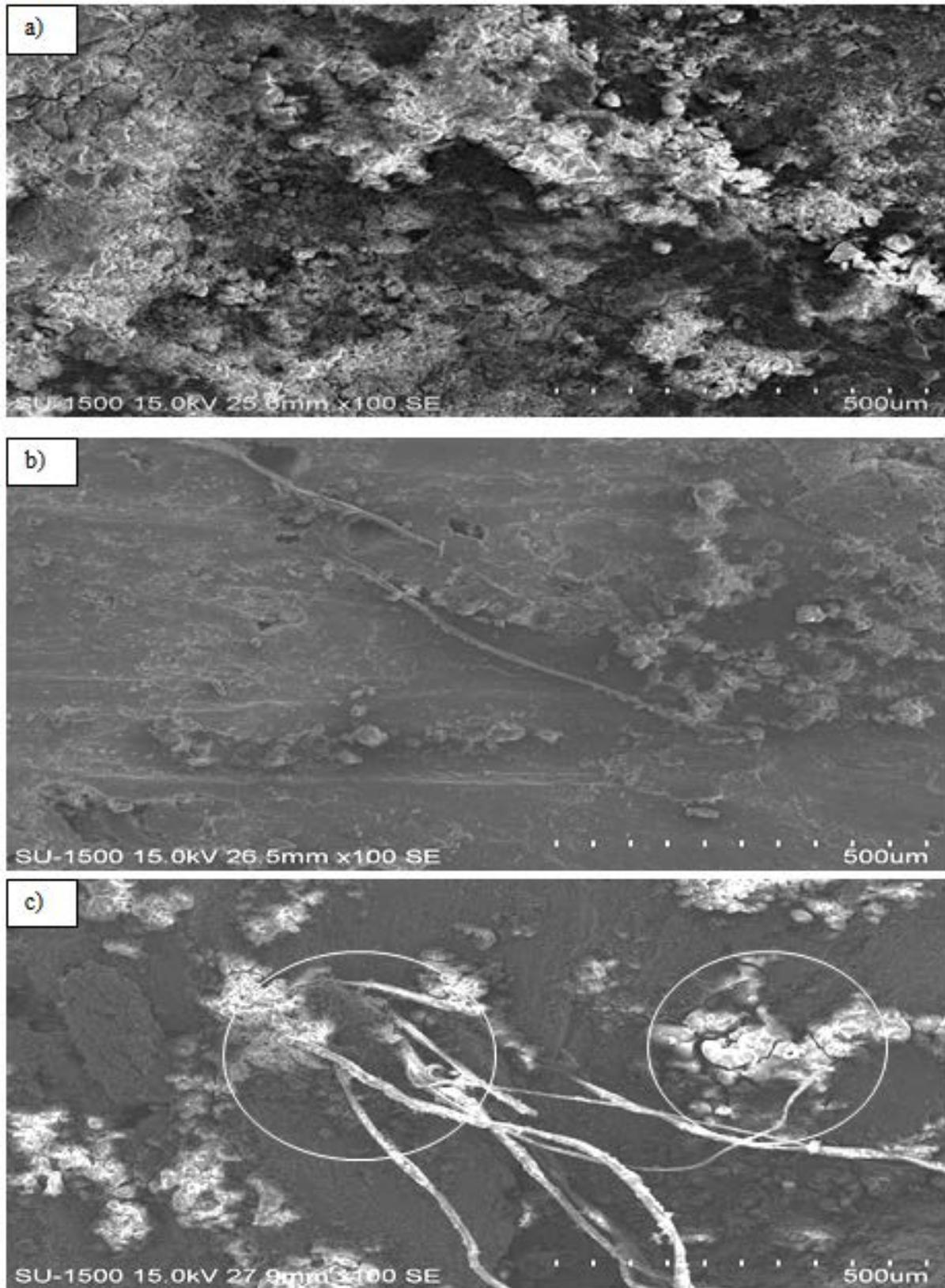
**Figure 3.** Shows corroded surface of the a) as cast Al7075 alloy, b) Al/ 5 wt. % of basalt short fiber and c) Al/ 10 wt.% of basalt short fiber composite
