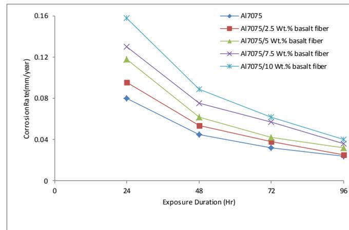
**Figure 1.** Corrosion rate of unreinforced matrix alloy and composites in 1 M HCl solution against exposure time
