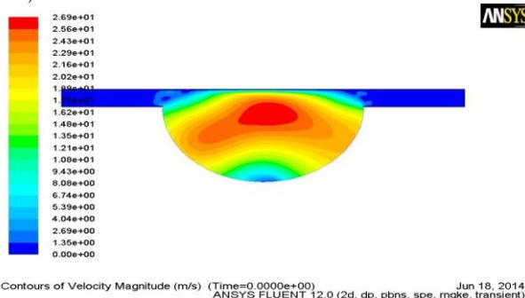
Figure 11. Gas velocity magnitude (m/s) CA = 360° (Max. Load) for biodiesel blend.
