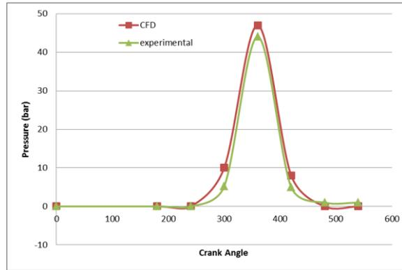
**Figure 4.** Comparisons between modeling and experimental pressure ( $p-\theta$ ) diagram of Biodiesel blend
