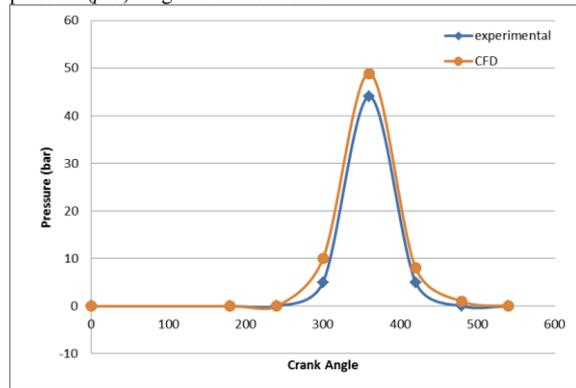
**Figure 5.** Comparisons between modeling and experimental pressure ( $p-\theta$ ) diagram of Diesel
