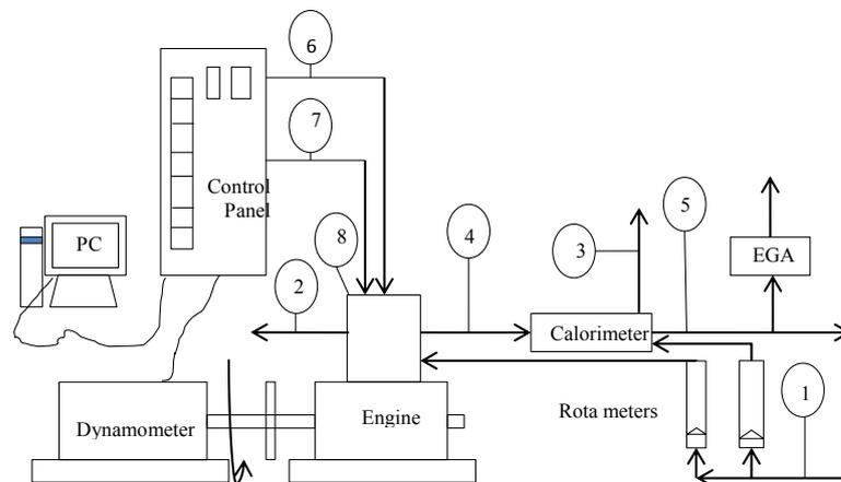
**Figure 1.** Schematic diagram of experimental set up.
