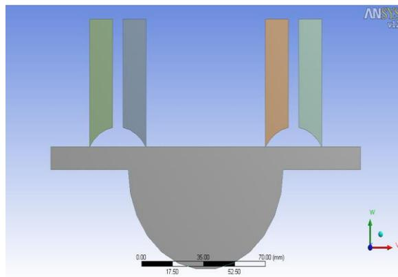
**Figure 2.** Geometry of combustion chamber with valves
