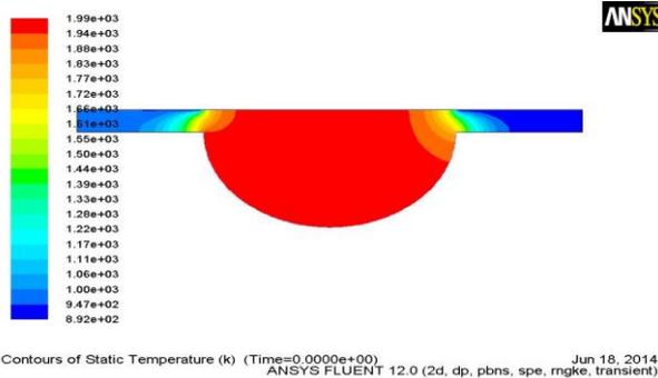
Figure 10. Temperature distribution in (K) CA = 360° (maximum load) for biodiesel blend
