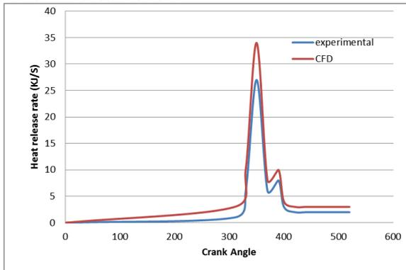
Figure 9. Comparison between modeling and experimental heat release rate for Diesel
