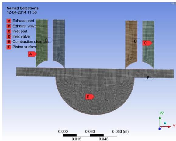
**Figure 3.** Mesh structure of computational domain for model geometry
