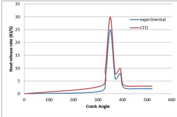
Figure 8. Comparison between modeling and experimental heat release rate for biodiesel blend
