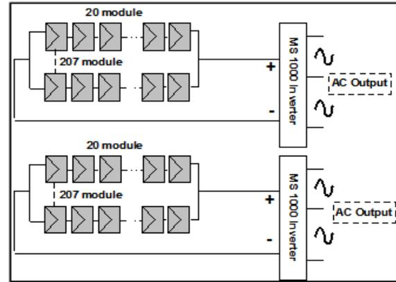
Figure 5 The array configuration of the central inverter
