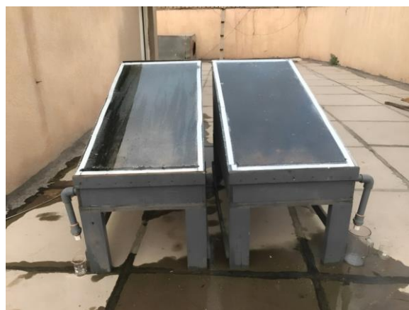
Figure 2. Photographic diagram of the solar water distillation apparatus
