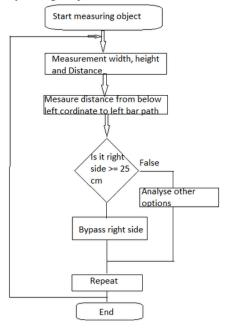
Figure 1. Flow Chart describing logic implementation [46]
