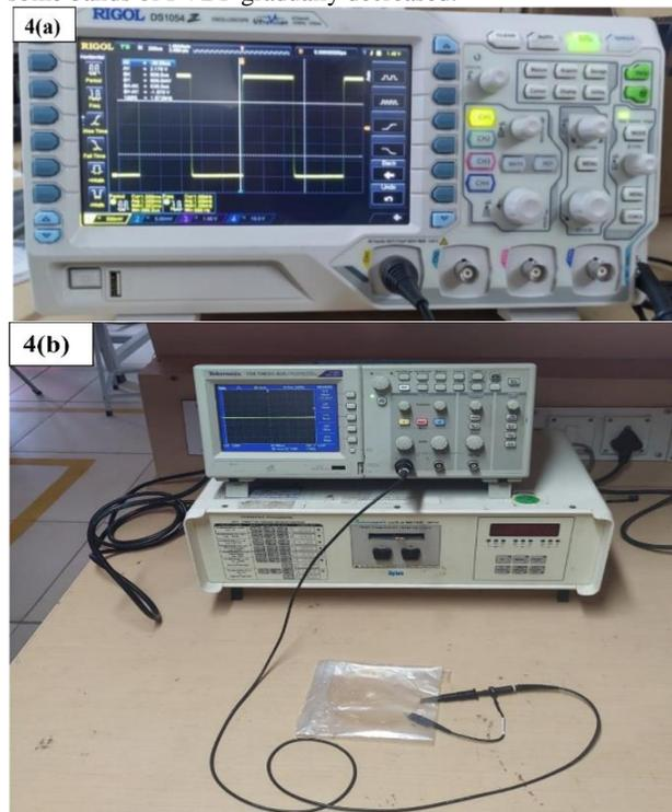
**Figure 4.** (a)Four-probe Digital Storage Oscilloscope (DS1054Z), (b) PVDF connected to Digital Storage Oscilloscope.
