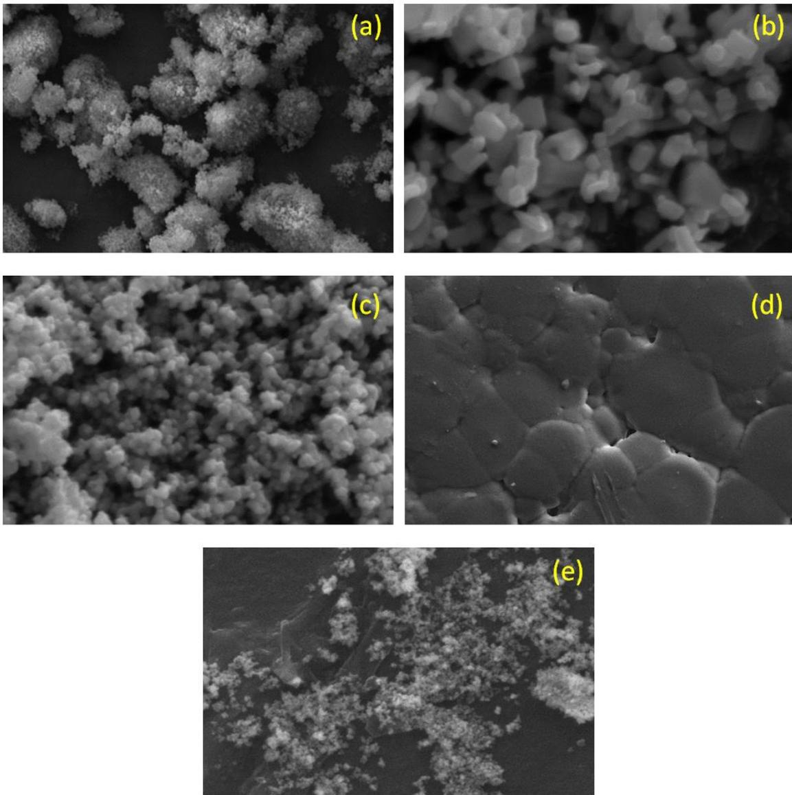
**Figure 5.** (a) 5(b) and 5(c) SEM images of PVDF, ZnO and TiO<sub>2</sub> nanofillers, (d) and 5(e) SEM images of neat PVDF films and 0.8wt.% ZnO and TiO<sub>2</sub> PVDF nanofilms
