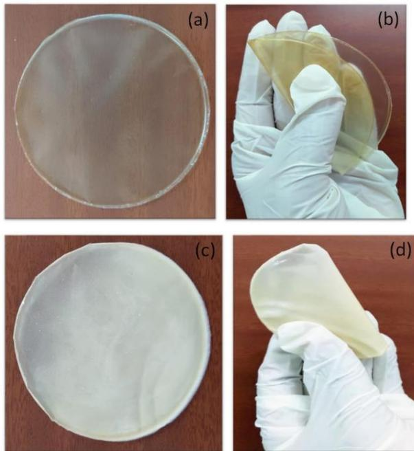
Figure 3. (a) and (b) Images of PVDF neat film and twisting of the film to confirm its, (c) and 3(d) Images of PVDF Nano film containing 0.2wt.% of ZnO and TiO<sub>2</sub> and twisting of the film to confirm its flexibility.
