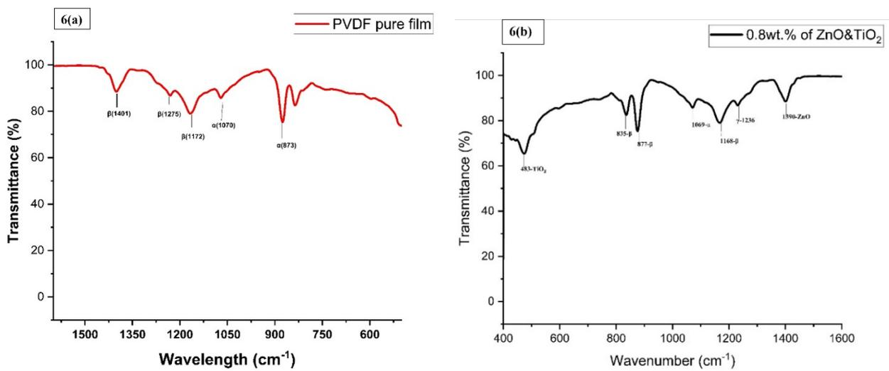
**Figure 6.** (a) FTIR spectra of PVDF film and (b) PVDF/0.8wt.% ZnO and TiO<sub>2</sub>
