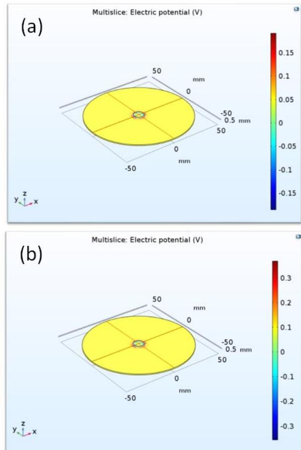
Figure 9. (a) and 9(b) images show the stimulated result for neat PVDF film and PVDF with 0.8 wt. % of ZnO and TiO<sub>2</sub> nanofillers
