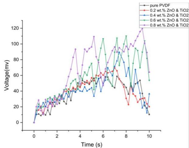
Figure 8. shows the Voltage Vs Time graph of neat PVDF film. and 0.2, 0.4, 0.6 and 0.8wt.% of ZnO and TiO<sub>2</sub> nanofilms.
