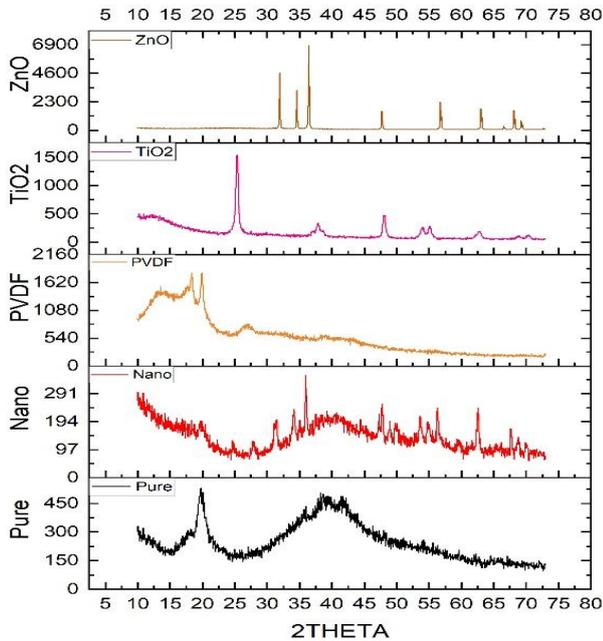
Figure 7. XRD spectra of nanofillers and PVDF nanofilms
