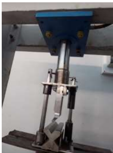
1- Punch guide sleeve, 2- Die, 3- Punch, 4- Guide shaft, 5- Base support, 6- Displacement control shims, 7- Sheet metal
