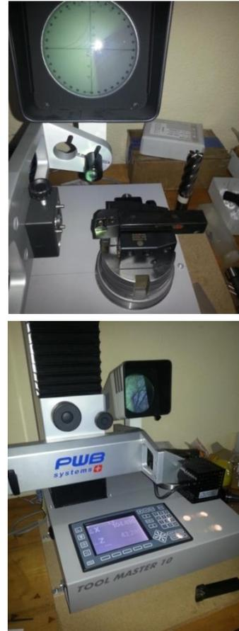
**Figure 3.1.** Equipment for measurement wears TOOL MASTER 10.
