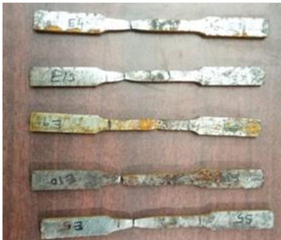
Figure 5. Tensile specimen after testing
