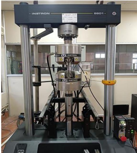
Figure 4. Instron UTM machine used for tensile test
