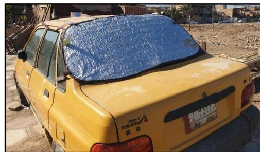
Figure 9. The external cover above the windshields.
