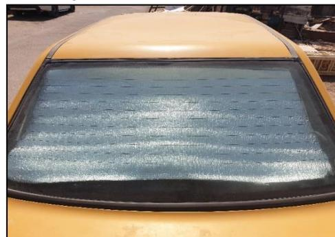
Figure 11. The internal cover beneath the windshields.
