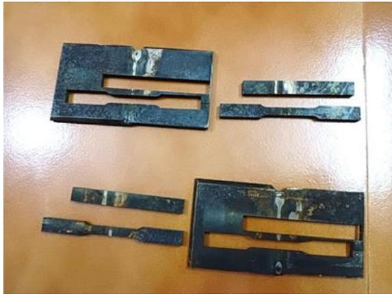
Figure 3. Specimen preparation for tensile test
