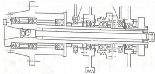
Figure 6. Schematic diagram of the spindle
