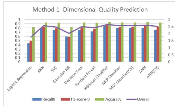
Figure 16. Plot for Dimensional accuracy using different ML techniques
