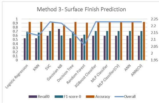
Figure 18. Plot for Surface finish prediction using different ML techniques- method 3
