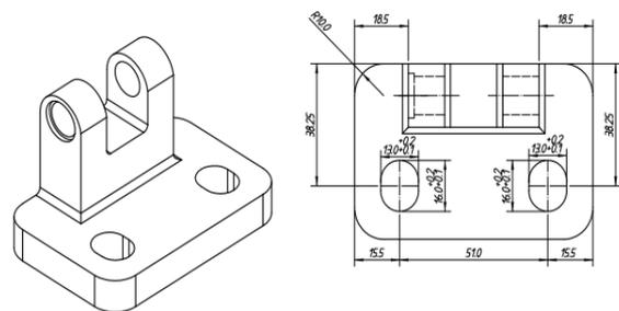
Figure 4. Hinge Type A
