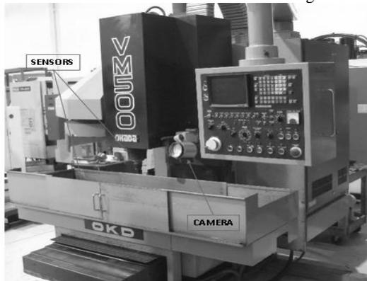
Figure 5. OKADA VM500 machine with sensors and cameras
