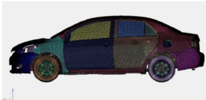
Figure 11. Finite element model of vehicle
