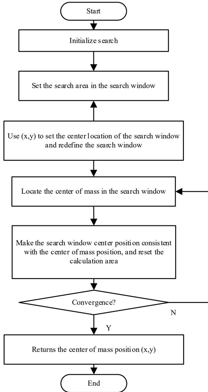
Figure 2. Tracking process based on Parallel Computing
