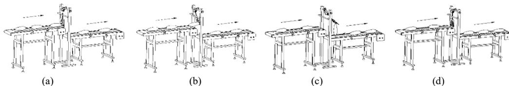
Figure 5. The process diagrams of orientation device when small diameter of the corn was in the front
