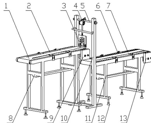
**Figure 1.** Three-dimensional modeling diagram of corn orientation device
