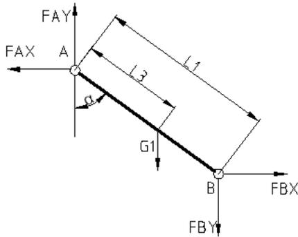
Figure 9. Stress analysis diagram of swinging rod
