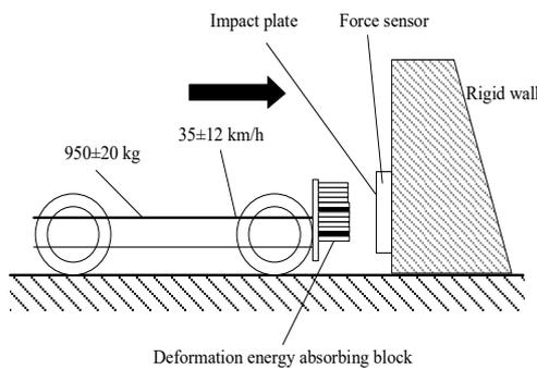
**Figure 4.** Schematic diagram of mobile barrier verification test
