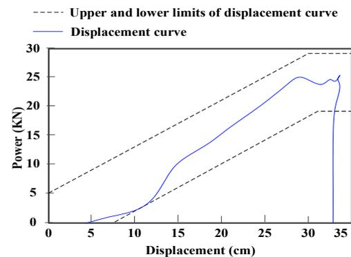
Figure 9. Force displacement curve of the fourth block
