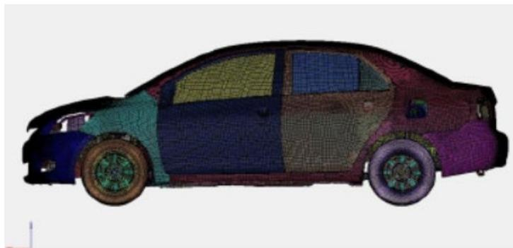
Figure 11. Finite element model of vehicle
