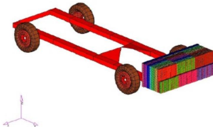
Figure 3. Finite element model of moving deformable barrier
