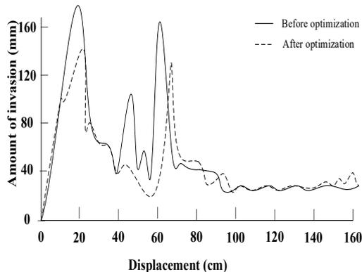
**Figure 16.** Comparison of B-pillar (chest position) invasion before and after optimization
