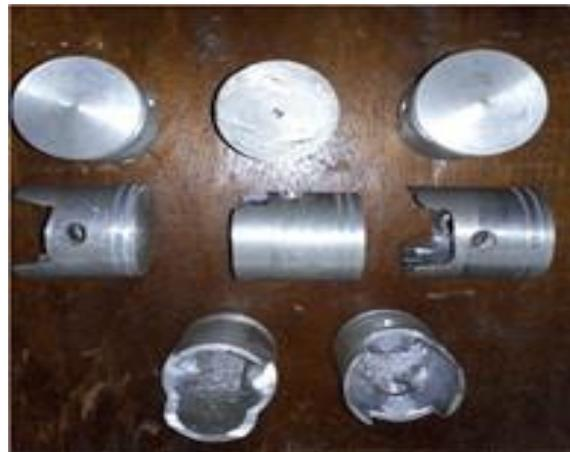
Figure 10. Machined cast pistons
