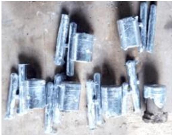
Figure 9. Unmachined cast pistons
