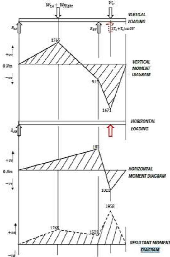
Figure 12. Bending moment diagram for the conveyor
