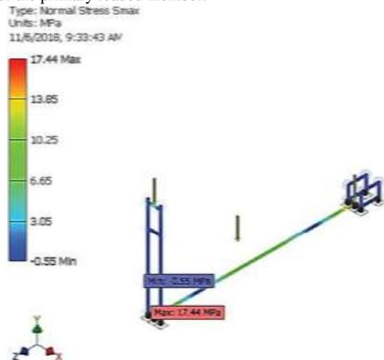
Figure 15. Normal Stress induced in the Frame.
