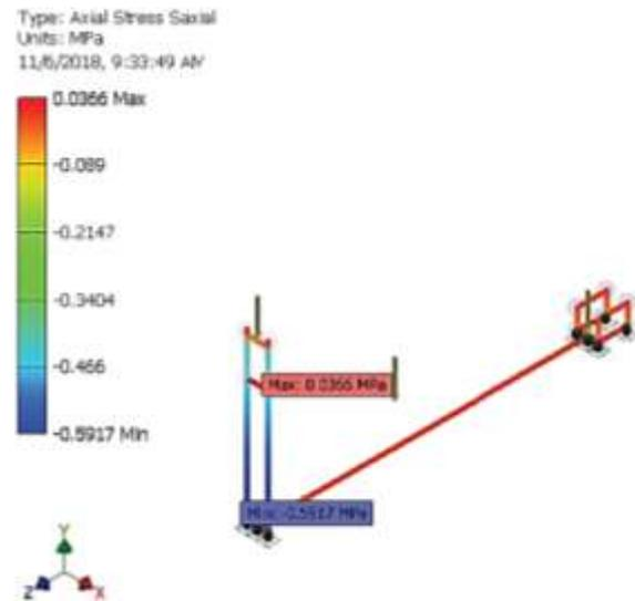
Figure 16. Axial Stress induced in the frame
