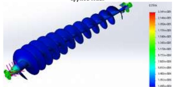
Figure 20. Equivalent Strain of the shaft under loads
