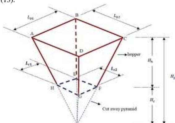
Figure 7. Schematic diagram of the hopper
