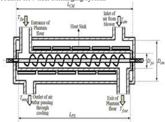
Figure 13. Schematic Diagram of the screw conveyor
