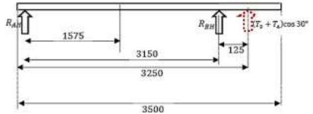
Figure 11. Horizontal Loading of the Screw shaft
