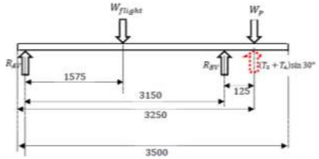
Figure 10. Vertical loading of the screw shaft
