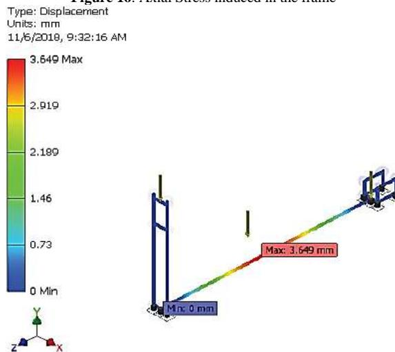
Figure 17. Displacement of frame members
