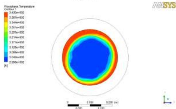
Figure 23. Contour showing flour outlet temperature distribution in the radial direction
