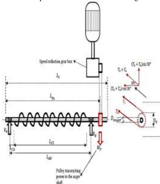
Figure 9. Drive and tail shafts assembly for the screw conveyor
