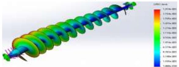
Figure 19. Displacement of the various nodes of the shaft under applied loads
