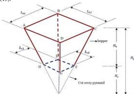
Figure 7. Schematic diagram of the hopper
