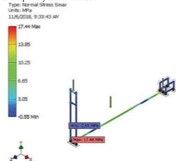
Figure 15. Normal Stress induced in the Frame.
