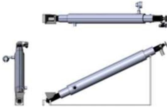
Figure 4. Orthographic view of the screw conveyor
