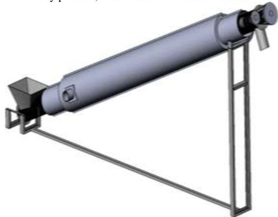
Figure 2. Isometric view of the screw conveyor
