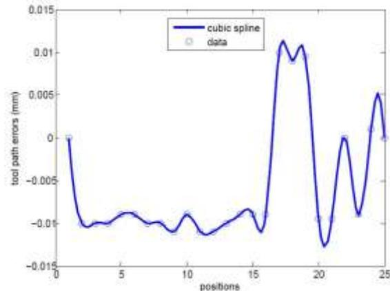
Figure 1. Cutting tool path error curve
