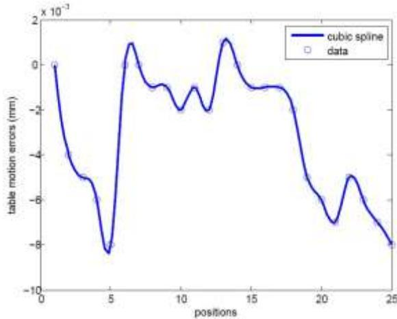
Figure 2. Table motion errors curve
