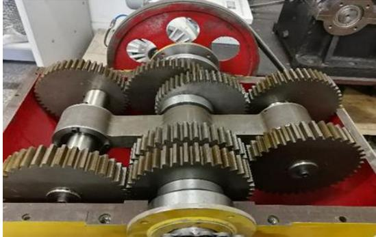
Figure 1. Reversing device of planetary gear train with elliptical cylindrical gears
