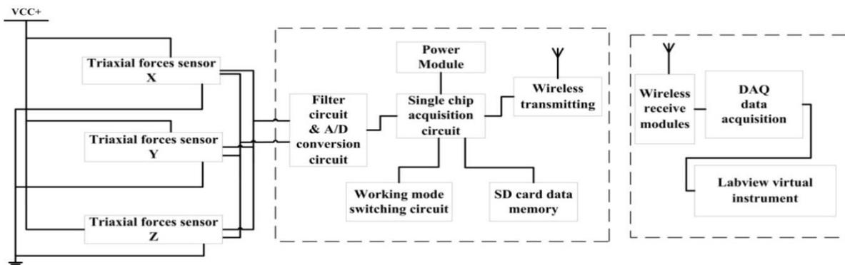
Figure 3: Embedded wireless testing system hardware diagram
