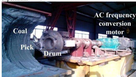
Figure 1: Coal cutting experiment and test system
