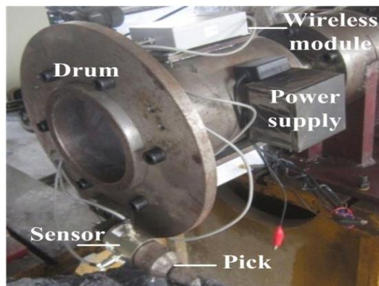
Figure 4: Pick sensor and wireless data transmission module
