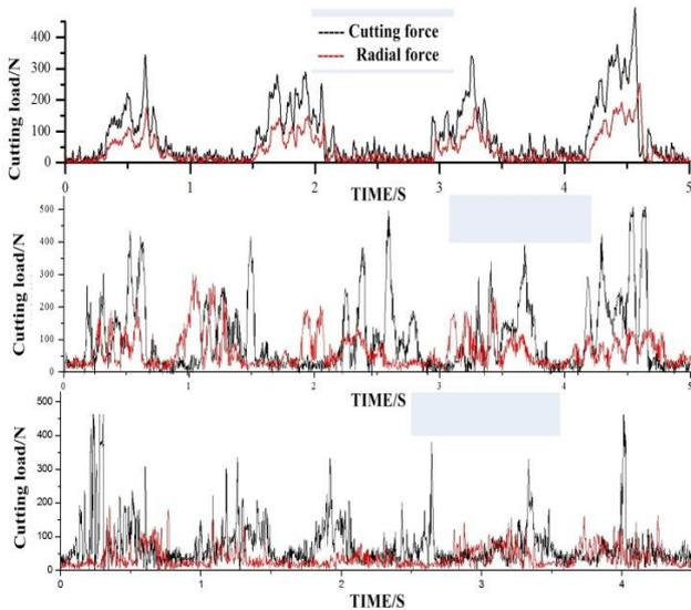
Figure 10: Time domain graph of cutting load with the drum rotating being 60r/min
