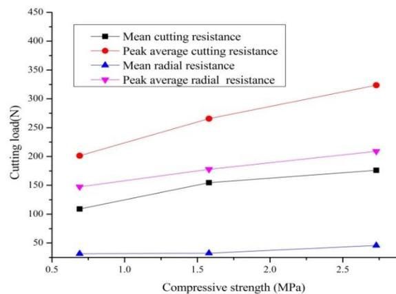
**Figure 7:** Relations of compressive strength and cutting force
