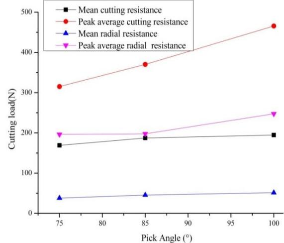
Figure 9: Relationship between pick-tip cone angle and cutting load
