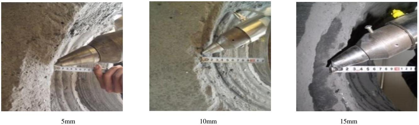
Figure 12: Presentation of different cutting thicknesses tests
