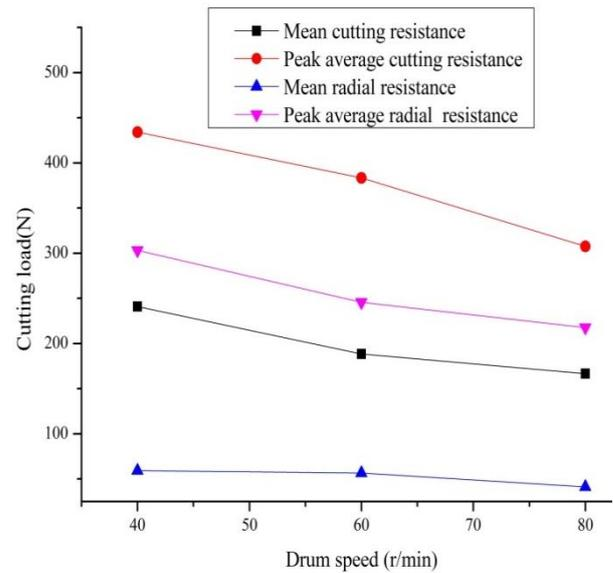
Figure 11: Relationship between drum rotating speed and cutting load
