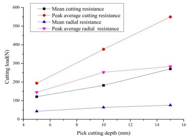
Figure 14: Relationship between cutting thickness and cutting load
