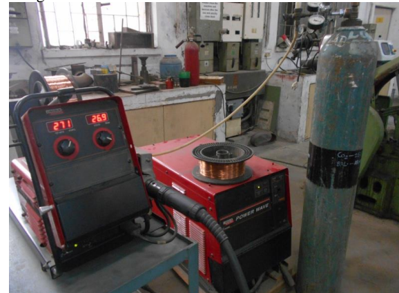
Figure 1: Actual welding setup of GMA
