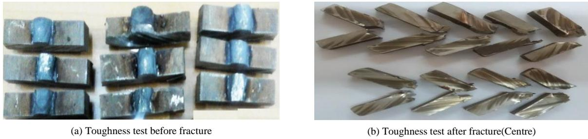
Figure 7: Toughness test samples
