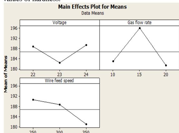
Figure 5: Main Effects Plot for SN ratios (VHN)
