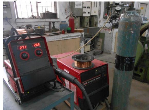
**Figure 1:** Actual welding setup of GMA
