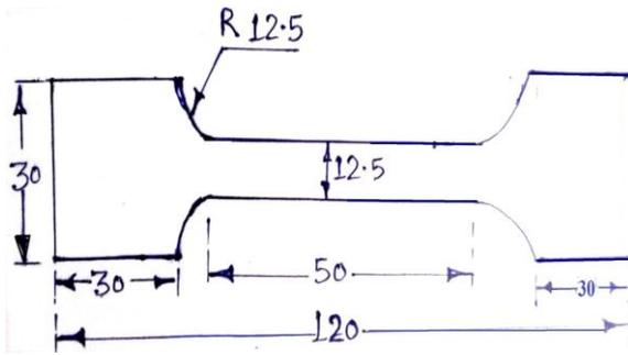
Figure 2: Tensile test specimen as per ASTM [12]
