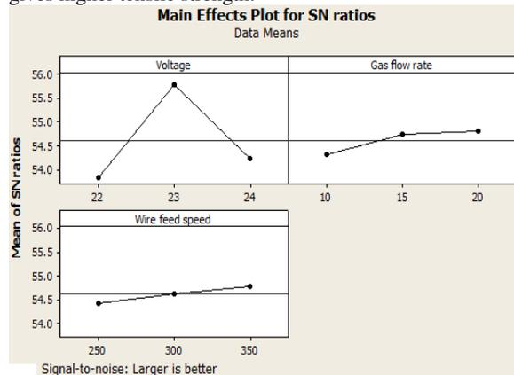
Figure 4: Main Effects Plot for SN ratios (UTS)
