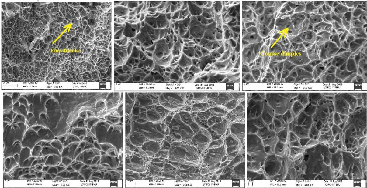
Figure 6: Fractograph morphology (SEM) of tensile test specimens
