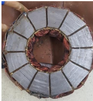
Figure 2. Stator consists of core and armature
