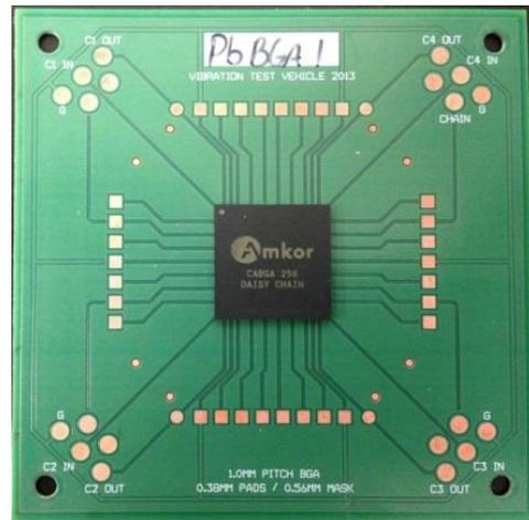
Figure 1. Test Board Details.
