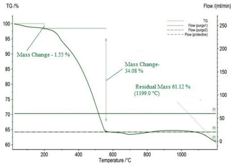
Figure 3. AF-22 brake material thermal analysis
