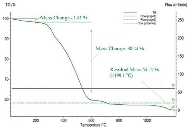
Figure 4. CL-3003 brake material thermal analysis
