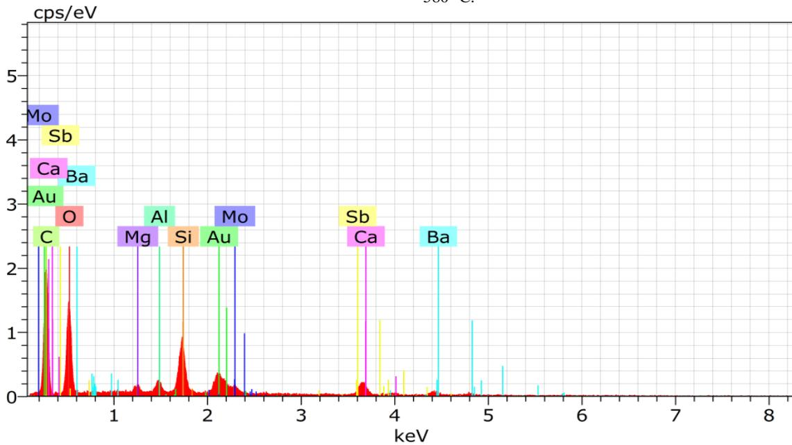
Figure 1. EDS spectrum for AF-22 brake pad material sample as detected
