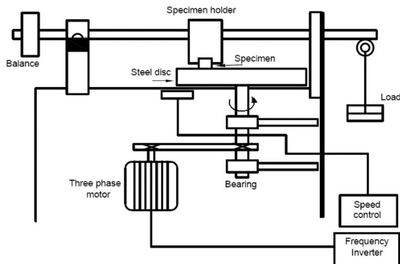
**Figure 5.** Pin-on-disc set-up
