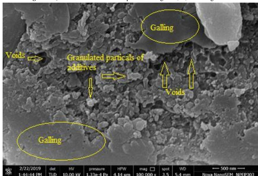
Figure 9. b) CL-3003 brake pad material sample SEM image at 1,00,000 x magnification
