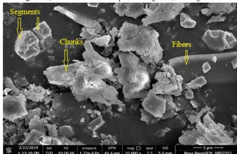
Figure 8. b) CL-3003 brake pad material sample SEM image at 10,000 x magnification
