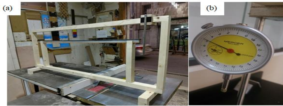
Figure 2. Experimental setup (a) main frame (b) dial gage.
