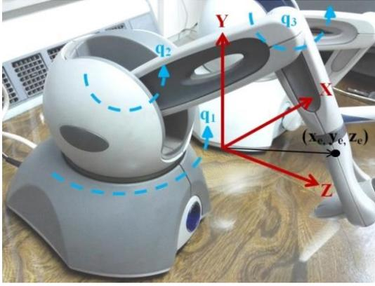
**Figure 4.** Phantom Omni reference XYZ coordinates, joints  $q_i$  and their resulting translational DoFs.
