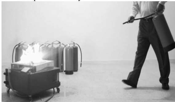
Figure 2. Third generation prototype of the Honeycomb fire simulator, and training extinguishers
