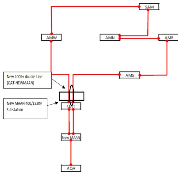
**Figure 6.** Current Jordanian 400kV grid structure with the reinforcements in the southern part
