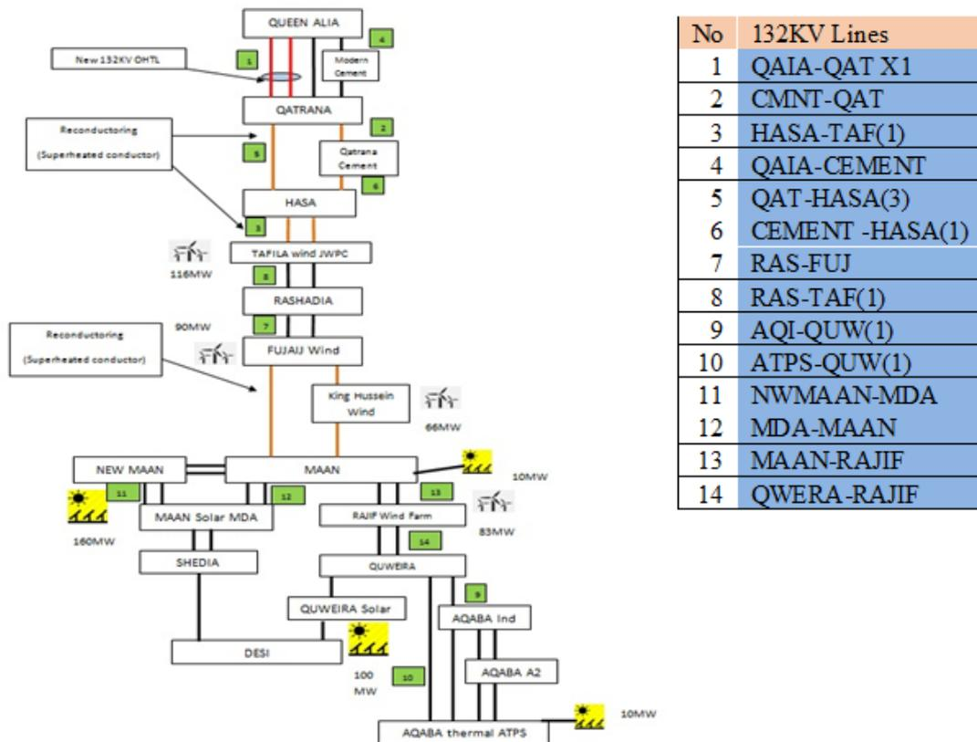
**Figure 4.** The connection of renewable projects in southern area in 2018 with reinforcement in the 132KV grid
