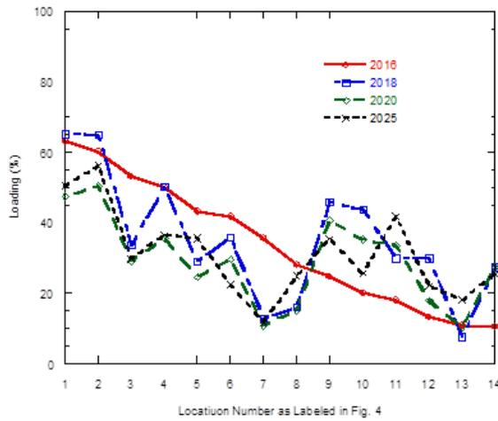
**Figure 5.** Loading of the 132KV lines in the southern part of Jordan with "Green Corridor"
