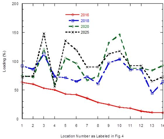
**Figure 3.** Loading of the 132KV lines in the southern part of Jordan using current grid
