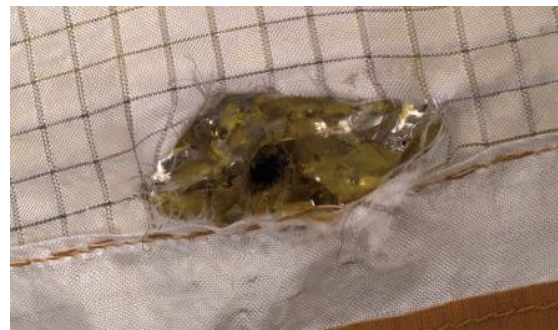
Figure 2. Detail of the damaged outer cover of the International Space Station
