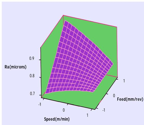
**Figure 7a.** Surface roughness vs Speed and Feed
