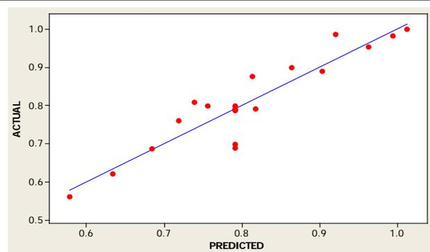
**Figure 4.** Scatter plot of  $R_a$  (actual Vs predicted)
