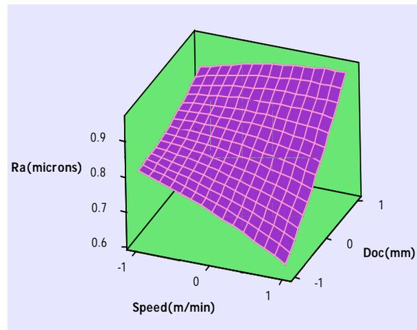
**Figure 7b.** Surface roughness vs Speed and Depth of cut
