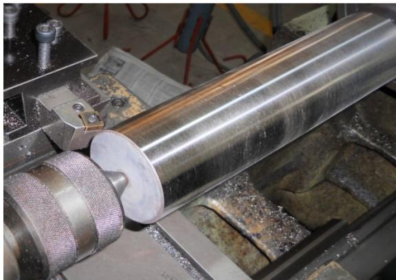
**Figure 8a.** Workpiece before machining
