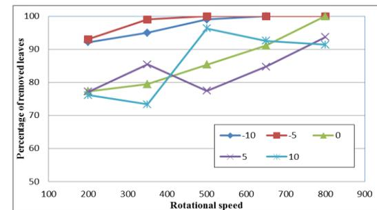
**Figure 6.** Effect of rotational speed on percentage of removed leaves for hardness 60 shor A.
