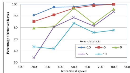
**Figure 5.** Effect of rotational speed on percentage of removed leaves for hardness 30 shor A.
