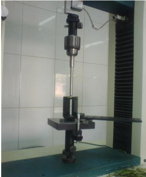
**Figure 2a.** Apparatus for the strength in bending experiment
