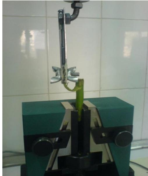
**Figure 2b.** Device to held and connect the leaf to UTM for picking force measuring
