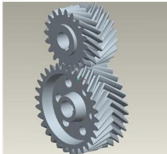
Figure 1. A pair of double helical gear
