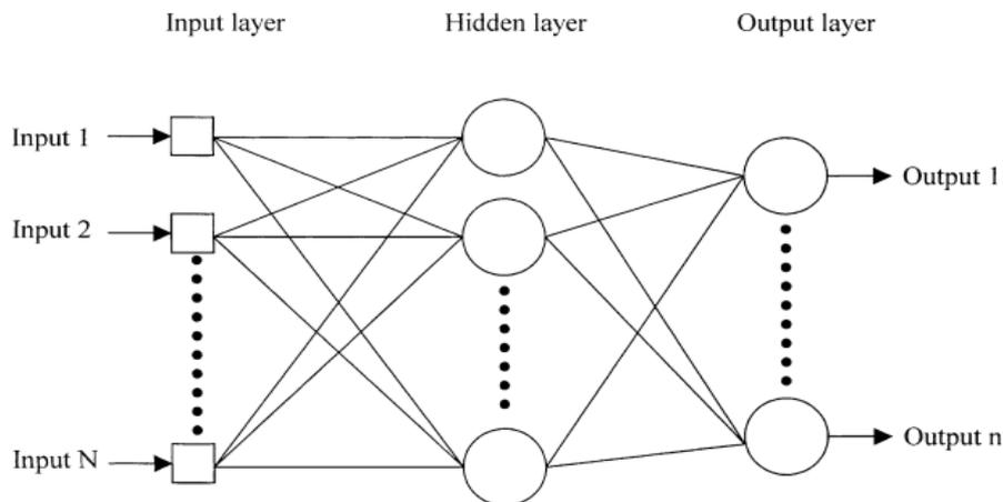
Figure 7. Multilayer feed forward network [29]
