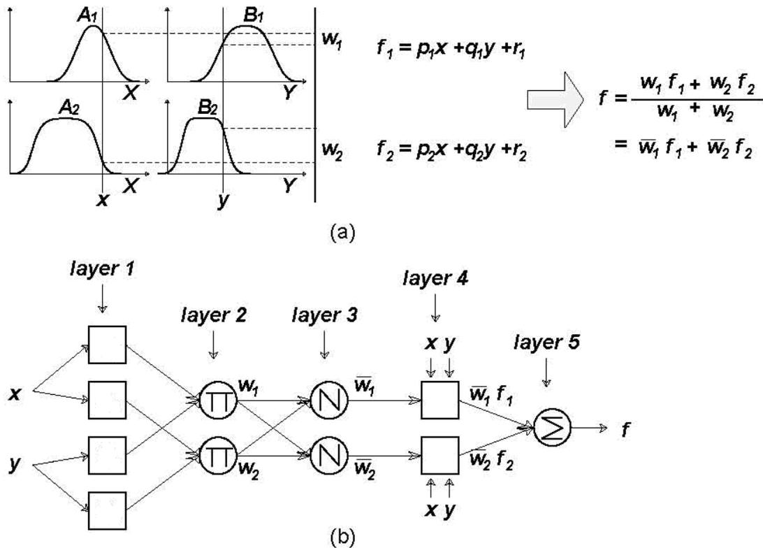
**Figure 4.** (a) Sugeno's FL system and (b) equivalent ANFIS [23]
