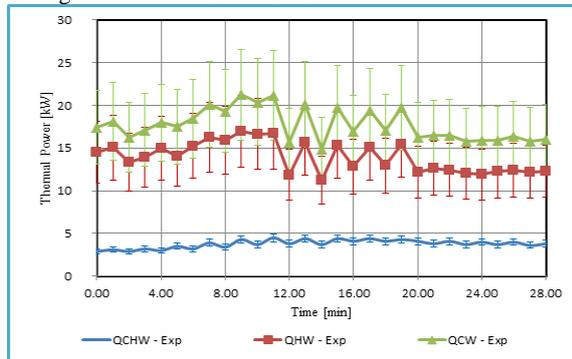
Figure 5. Chiller thermal powers and measurement uncertainties
