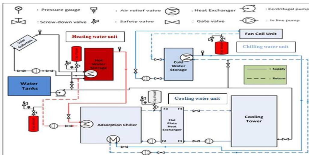
Figure 2. Schematic diagram of the solar powered adsorption chiller
