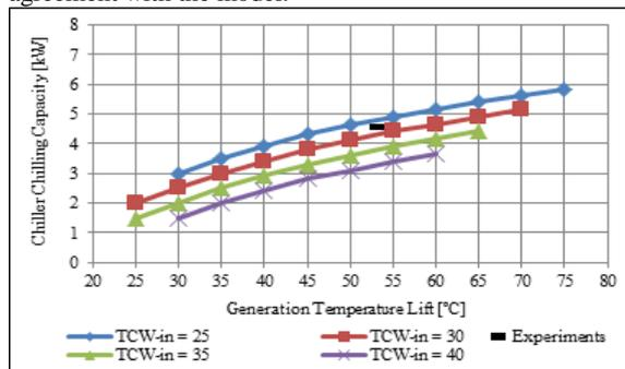
**Figure 9.** Generation temperature lift influence on chiller performance
