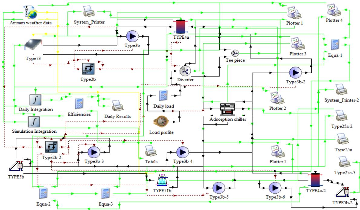
Figure 3. TRNSYS project for simulation of the solar adsorption system
