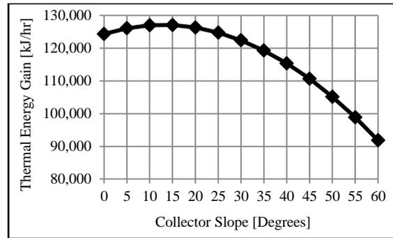
Figure 7. Thermal power gain for more different collector tilts
