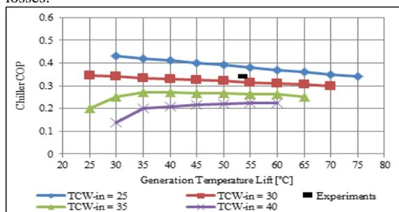
**Figure 10.** The influence of generation temperature lift on chiller COP
