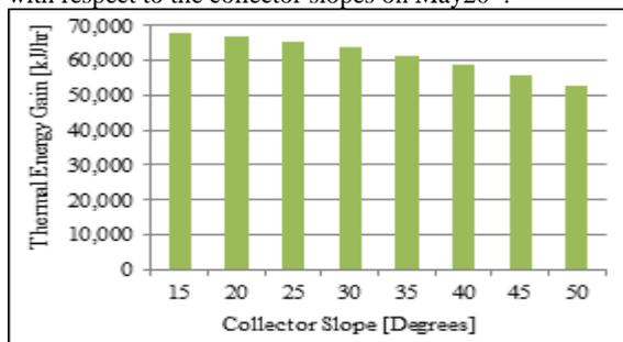
Figure 6. Collector thermal gain for different collector tilts (Simulations on May 20<sup>th</sup>)
