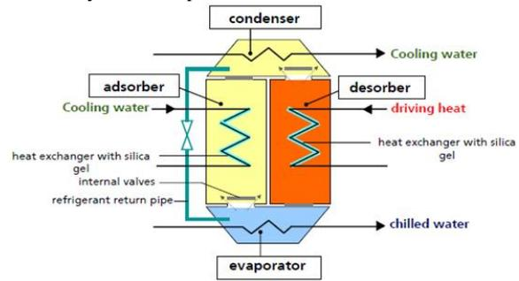
Figure 1. Schematic of adsorption cycle solar cooling system
