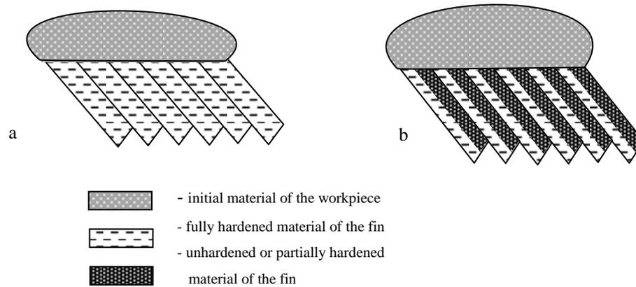
**Figure 6.** Modifications of structures obtained during quenching deformational cutting: a- fully hardened over the thickness of fin, c - partially hardened over the thickness of fin
