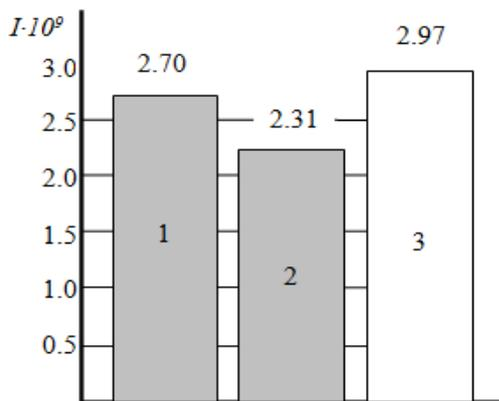
**Figure 10.** Wear intensity. Steel 40H. 1 – after DC without tempering, 2 – after DC with low-temperature tempering, 3 – after standard volumetric tempering with low-temperature tempering
