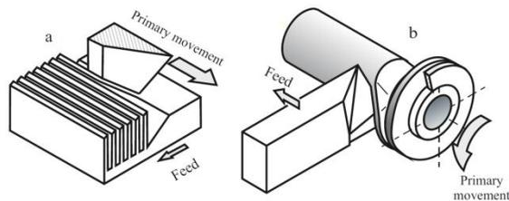
**Figure 1.** Concept of deformational cutting: shaping of flat surfaces (a), turning of cylindrical surfaces (b)
