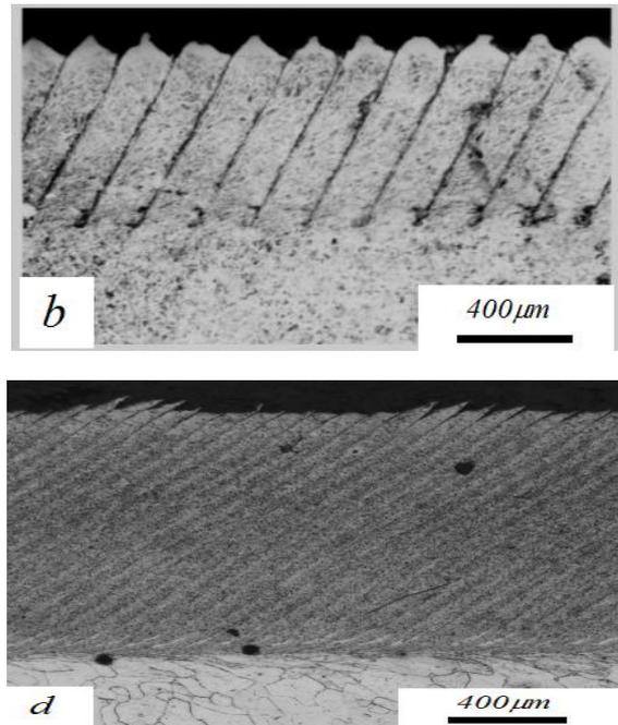
**Figure 5.** Examples of deformational cutting on steels with a zero interfin. a- steel 30HGSA,  $p = 0,4$  mm; b – steel 20KH13,  $p = 0,2$  mm; c – steel 35,  $p = 0,1$  mm; d - Armco iron,  $p = 0,1$  mm.
