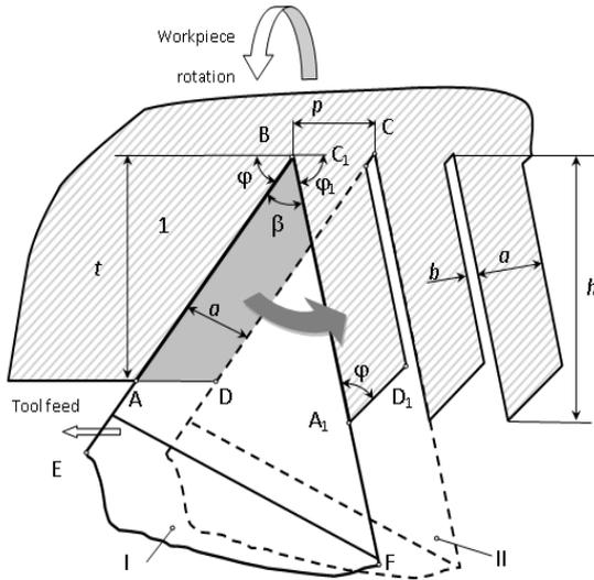
**Figure 4.** Fin shaping scheme by the deformational cutting method
