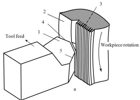
**Figure 2.** Concept of DC hardening. 1- DC tool, 2-surface to be hardened, 3 – hardened surface, 4 - cutting edge, 5 - deforming edge
