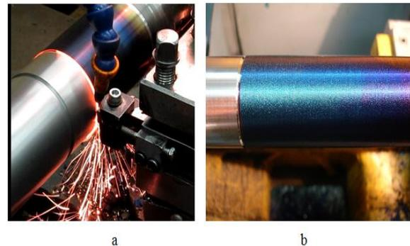
**Figure 3.** a - Process of DC hardening, b - hardened shaft
