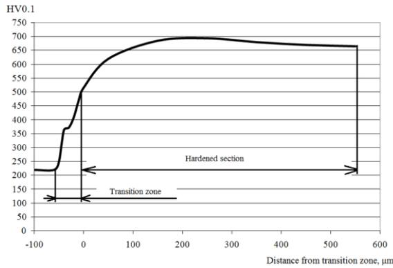
**Figure 8.** Distribution of microhardness over the thickness of the hardened layer. Steel 35, pitch of the structure  $p=0.05$  mm.
