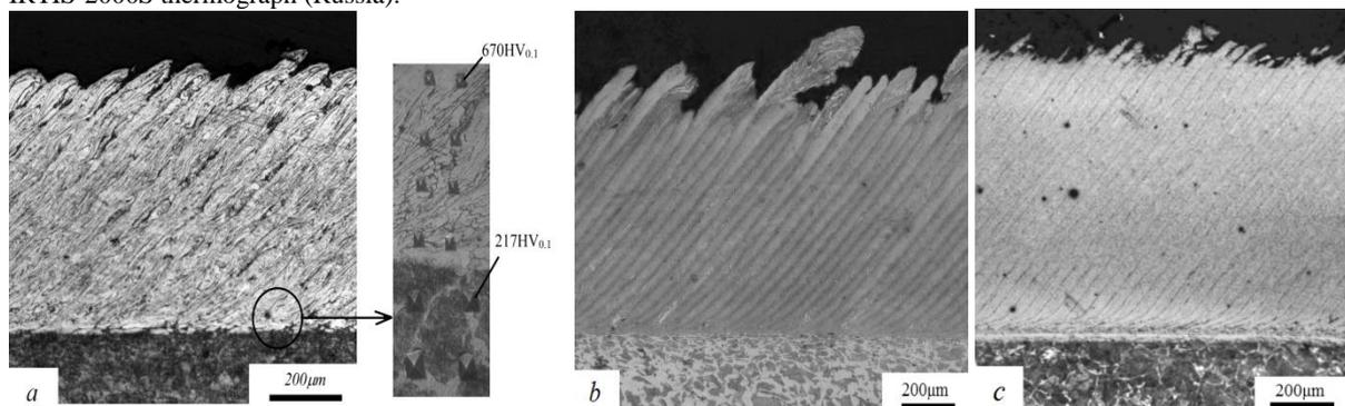
**Figure 7.** Total hardening over the thickness of fin. a- steel 35, pitch of the structure 0.15 mm,  $740HV_{0.1}$ , b - steel 35, pitch of the structure 0.05 mm,  $650HV_{0.1}$ , c - steel 40H, pitch of the structure 0.05 mm,  $680HV_{0.1}$ .
