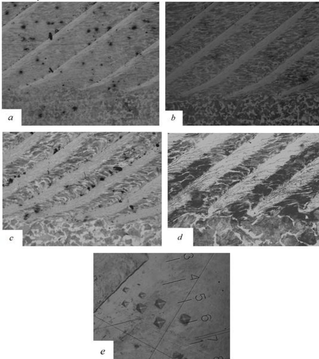
**Figure 9.** Hardened structures on steel 35 with various ratios of fully hardened and partially hardened material of fin. a - tool material ZM332,  $p=0.15$  mm, b - tool material SiAlON,  $p=0.1$  mm, c - tool material SiAlON,  $p=0.1$  mm, d - tool material CBN,  $p=0.1$  mm, e- comparison of dimensions of imprints in fully and partially hardened fin area
