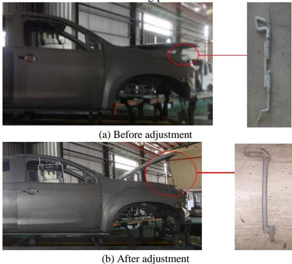
Figure 7. Repositioning of the bonnet
