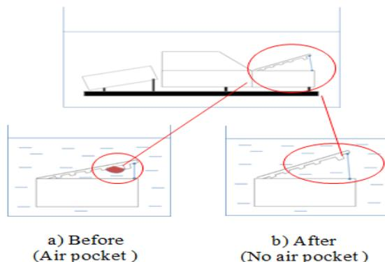
Figure 13. Bonnet's inner surface comparisons after bonnet adjustment
