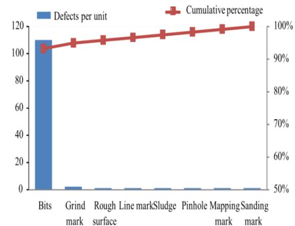
Figure 1. The electrodeposition defects
