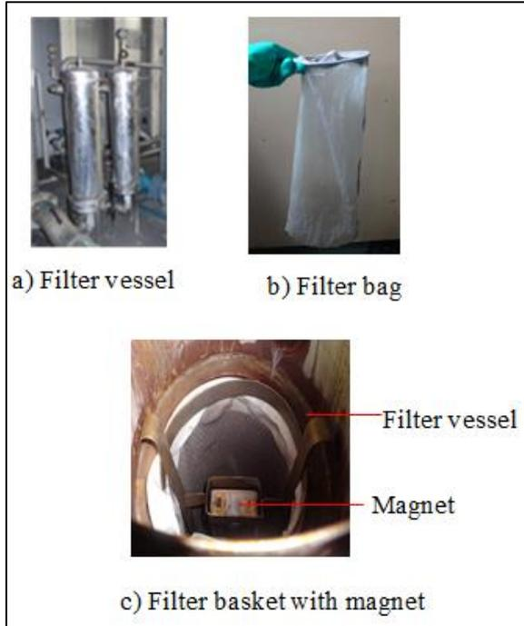
Figure 6. Filtration system with filter bag and magnet
