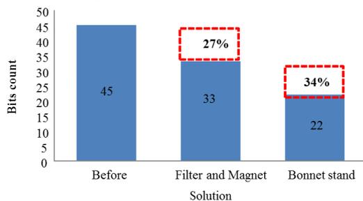
Figure 12. Bits count on unit after bonnet adjustment
