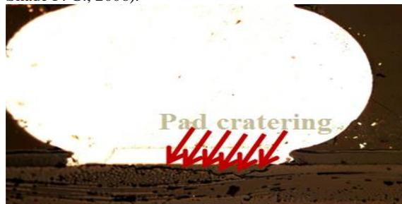
Figure 1. Pad cratering Failure mode
