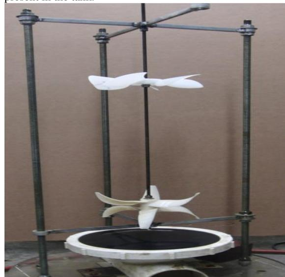
**Figure 4.** Supporting structure illustration
