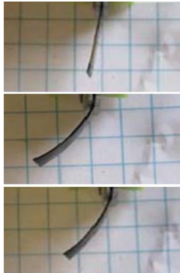
Figure 2. The deflections of the IPMC strips under a square wave, Specimen No. one
