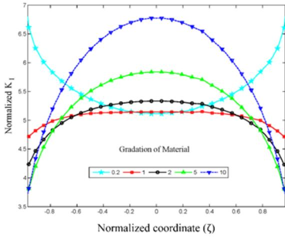
**Figure 6.** Distribution of the normalized  $K_I$  along the crack front in a rotating FGM cylinder with different values of material gradation for constant  $\eta = \xi = 0.4$ ,  $\nu = 0.30$  and diameter ratio (RD) of 1.5
