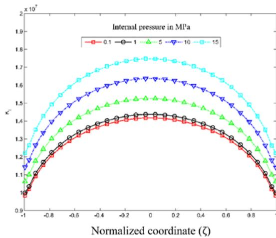
**Figure 8.** Variation of the  $K_I$  along the crack front for different internal pressure in a rotating FGM cylinder with  $\eta = \xi = 0.4$ ,  $RE=2$ ,  $RD=2$ .
