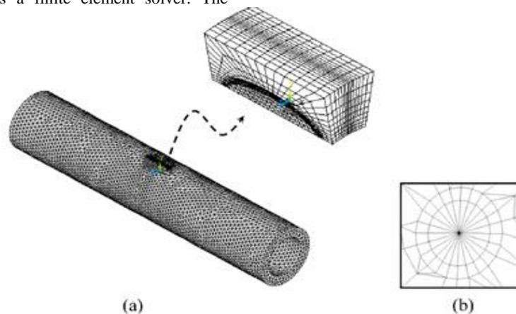
**Figure 2.** Finite element model of cylinder: (a) the whole model and the corresponding sub-model, (b) the singular elements near the crack front
