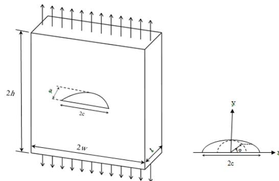
**Figure 3.** Semi-elliptical surface crack in a FGM plate under tension
