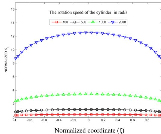
**Figure 9.** Variation of the normalized  $K_I$  along the crack front in a rotating FGM cylinder for different rotational speed with  $\eta = \xi = 0.4$ ,  $RE=2$ ,  $RD=2$ .
