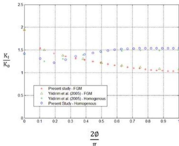
**Figure 4.** Variation of the normalized mode-I stress intensity factor on the crack front in a FGM plate with  $\xi = \frac{1}{3}$ ,  $\eta = 0.8$ ,  $\nu = 0.25$ ,  $E(r_o)/E(r_i) = 0.2$  and homogeneous material.
