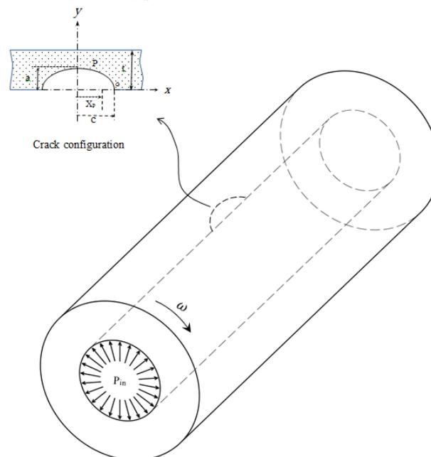
**Figure 1.** Longitudinal internal semi-elliptical surface crack in a rotating thick walled cylinder.
