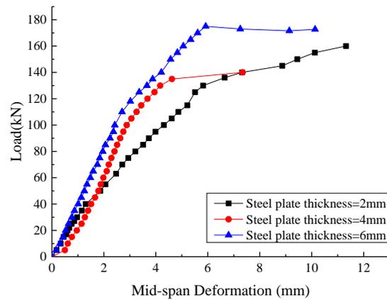
Figure 8. Load-mid-span deflection of beam with cover thickness=35mm
