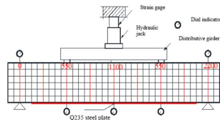
Figure 6. Test beam loading
