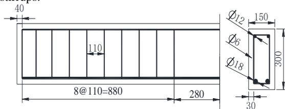
Figure 4. Test beam reinforcement drawing.
