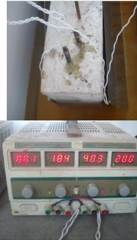
(1) Fast electrochemical corrosion
