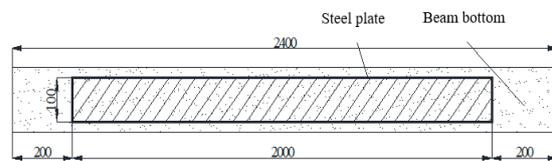
(2) Schematic diagram of bonded steel plate
