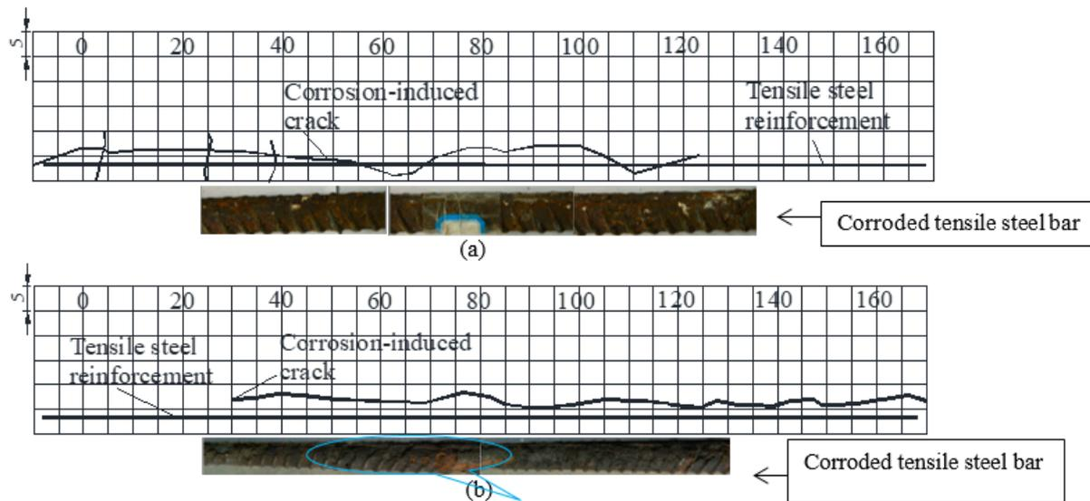
Figure 7. Corrosion-induced cracks distribution of the beam specimens and corrosion condition of tensile steel reinforcement: (a) P1; (b) P2
