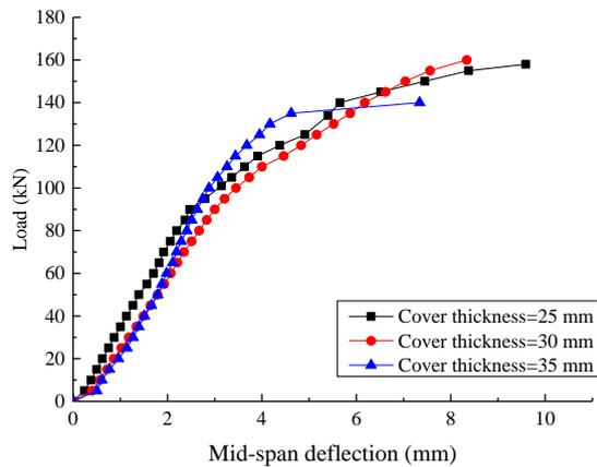
**Figure 9.** Load-mid-span deflection of beam with steel plate thickness=4mm
