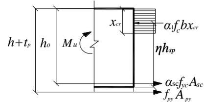
Figure 2. Forced section of the test beam after steel plate reinforcement.
