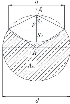
Figure 1. Model of steel bar with pitting corrosion.
