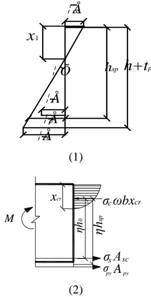
**Figure 3.** Stress distribution of simple bending section and mid-span section.
