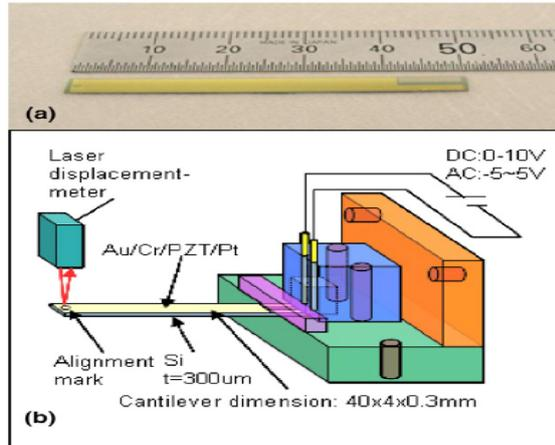
**Figure 4.** a) The prepared PZT cantilever, b) and the measurement setup of the microactuator.
