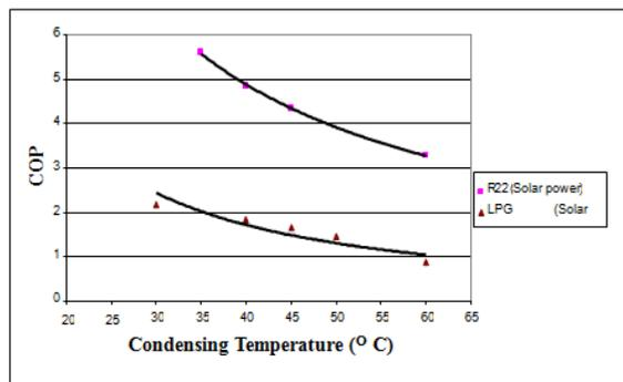
Figure 17: COP vs. Condensing Temperature for R22 and LPGM at  $T_e = 5\text{ }^\circ\text{C}$ .
