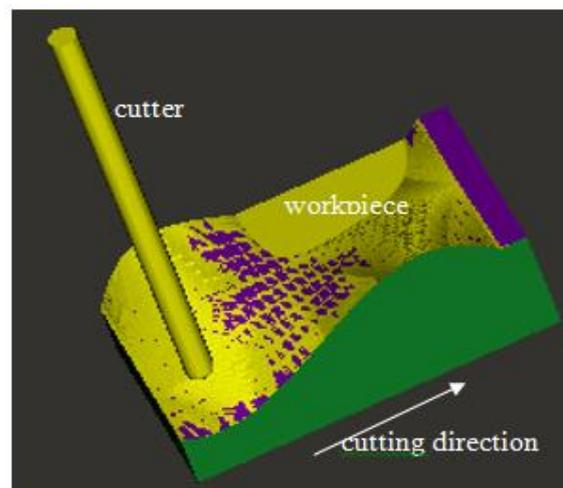
Figure 1: Free form surface created using end milling.
