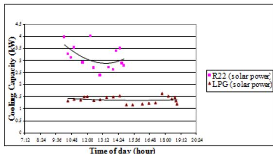
Figure 10: Cooling capacity using R-22 and LPGM.
