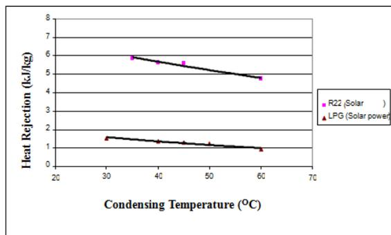
Figure 20: Heat Rejection vs. Condensing Temperature for R22 and LPGM at  $T_e = 5\text{ }^\circ\text{C}$ .
