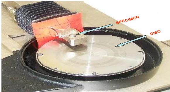
Figure 1: Test specimen on the tribometer disc.
