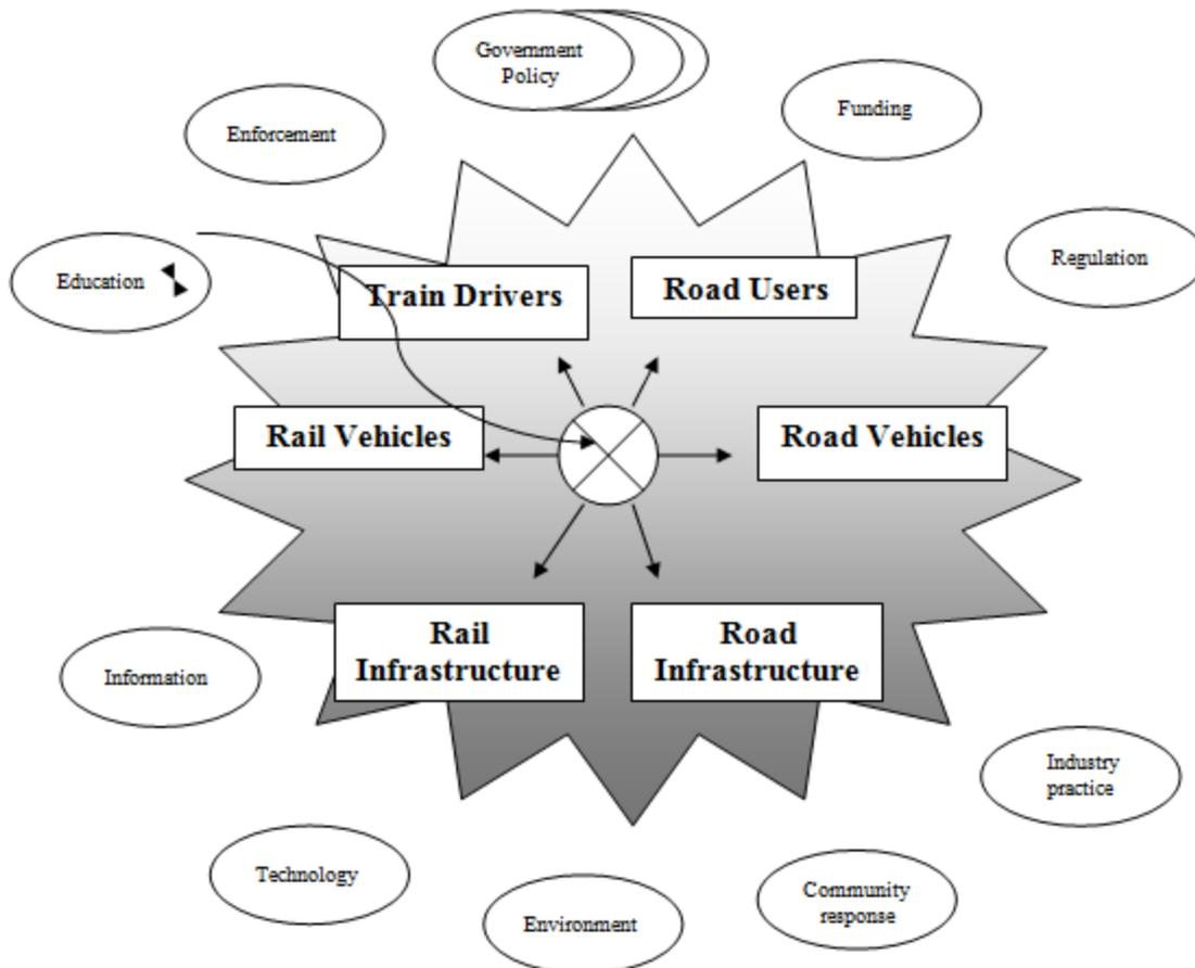
Figure 3: Components of railway level crossing safety.
