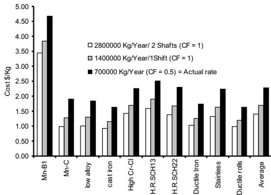
Figure 8: A comparison of cost of different alloy types under variant production rate based on ABC.
