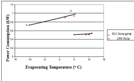
Figure 15: Power Consumption vs. Evaporating Temperature for R22 and LPGM at  $T_c = 45\text{ }^\circ\text{C}$ .
