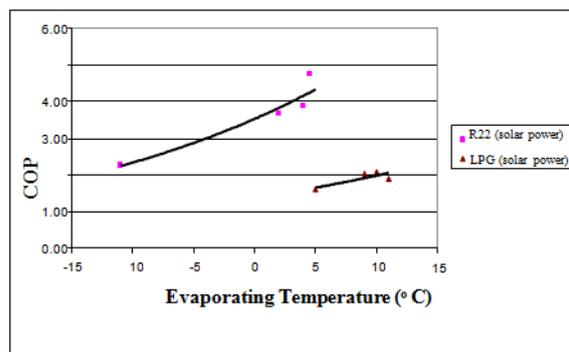
Figure 13: COP vs. Evaporating Temperature for R22 and LPGM at  $T_c = 45^\circ\text{C}$ .
