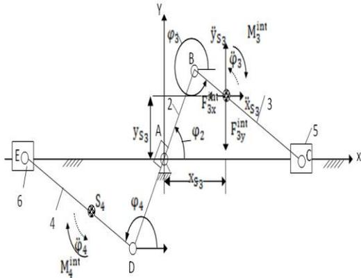
Figure 10: Self balanced slider – crank system.
