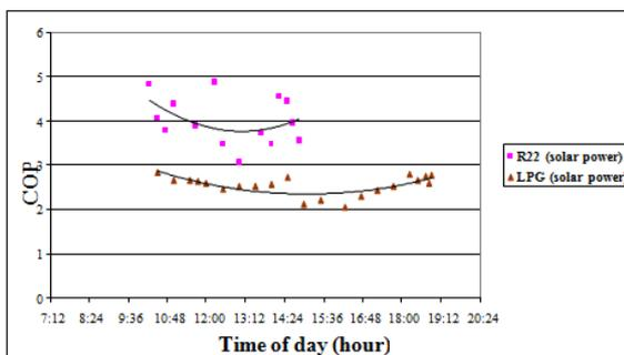
Figure 11: Coefficient of performance using R22 and LPGM.
