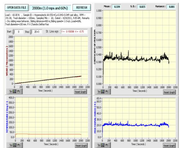
Figure 7: Data acquisition report of the specimen.
