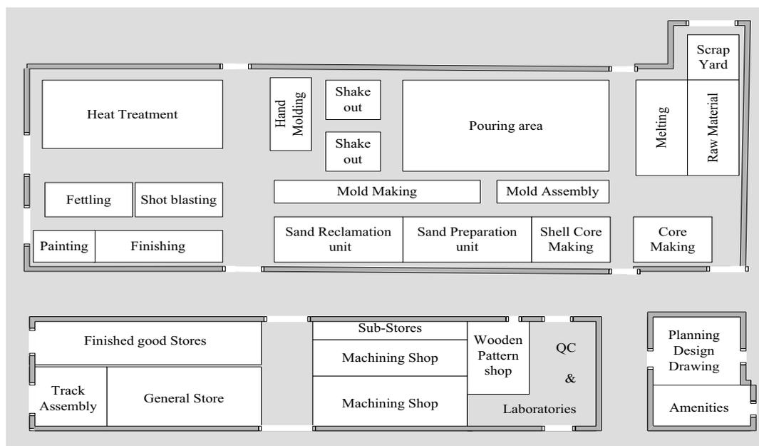
Figure1: Layout of the proposed steel foundry and its support departments
