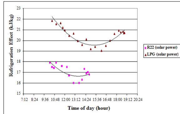
Figure 8: Refrigeration effect using R-22 and LPGM.
