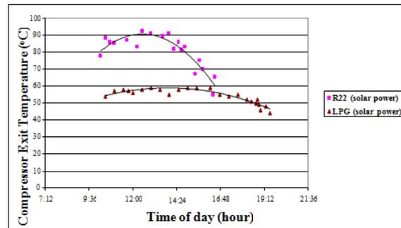
Figure 12: Compressor exit temperature with R22 and LPGM.
