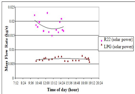
Figure 9: Mass flow rate using R-22 and LPGM.
