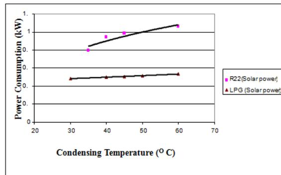
Figure 19: Power Consumption vs. Condensing Temperature for R22 and LPGM at  $T_e = 5\text{ }^\circ\text{C}$ .
