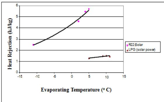
Figure 16: Heat Rejection vs. Evaporating Temperature for R22 and LPGM at  $T_c = 45\text{ }^\circ\text{C}$ .
