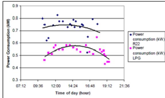
Figure 7: Power consumption using R-22 and LPGM.
