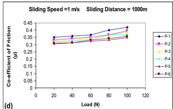
Figure 4: Variation of (a) wear volume (b) volumetric wear rate (c) wear resistance (d) coefficient of friction, with different loads at 1 m/s sliding speed and 1000m sliding distance.
