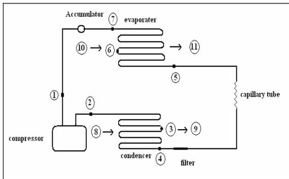
Figure 2: Temperature measuring location of the test air conditioning.
