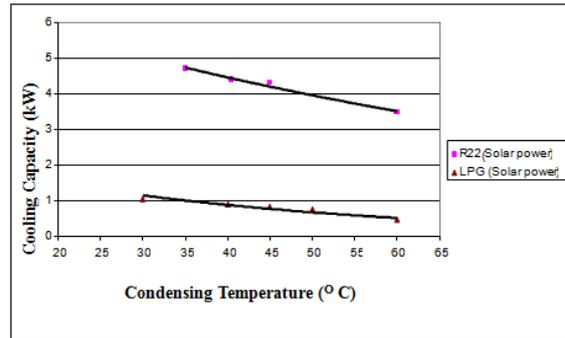
Figure 18: Cooling Capacity vs. Condensing Temperature for R22 and LPGM at  $T_e = 5\text{ }^\circ\text{C}$ .
