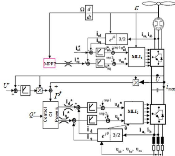
Figure 4: Global diagram of the permanent magnet synchronous generator control.
