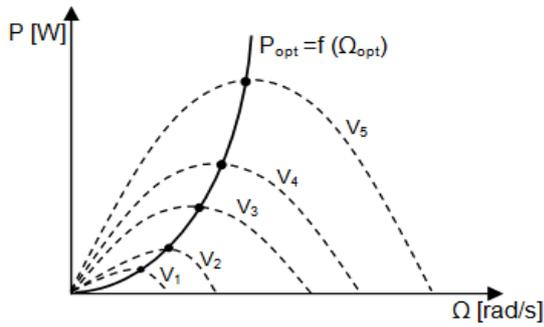
Figure 2: Feature of wind turbine in the plan power, rotational speed.
