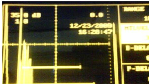
Figure 12: Sample 2 subsurface defects using UT at PR = 6.3 (cm<sup>3</sup>/s).
