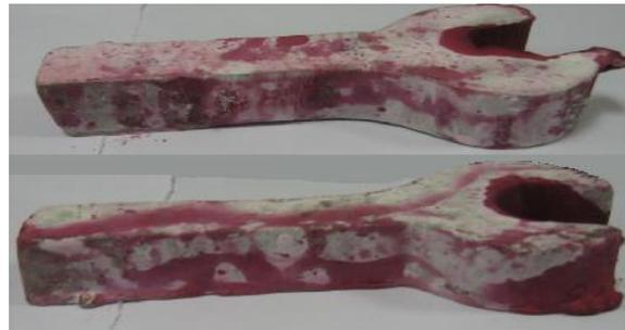
Figure 4: Sample 4 surface defects using PT at PR = 9.4 (cm<sup>3</sup>/s).
