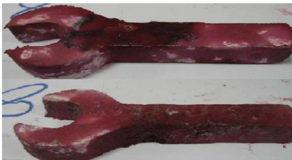
Figure 10: Sample 10 surface defects using PT at PR = 24 (cm<sup>3</sup>/s).
