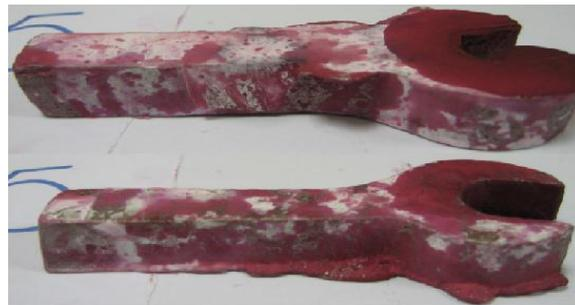
Figure 5: Sample 5 surface defects using PT at PR = 12.6 (cm<sup>3</sup>/s).
