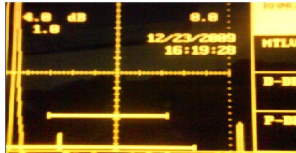
Figure 20: Sample 10 subsurface defects using UT at PR = 24 (cm<sup>3</sup>/s).
