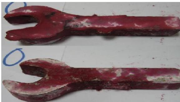
Figure 9: Sample 9 surface defects using PT at PR = 19.2 (cm<sup>3</sup>/s).
