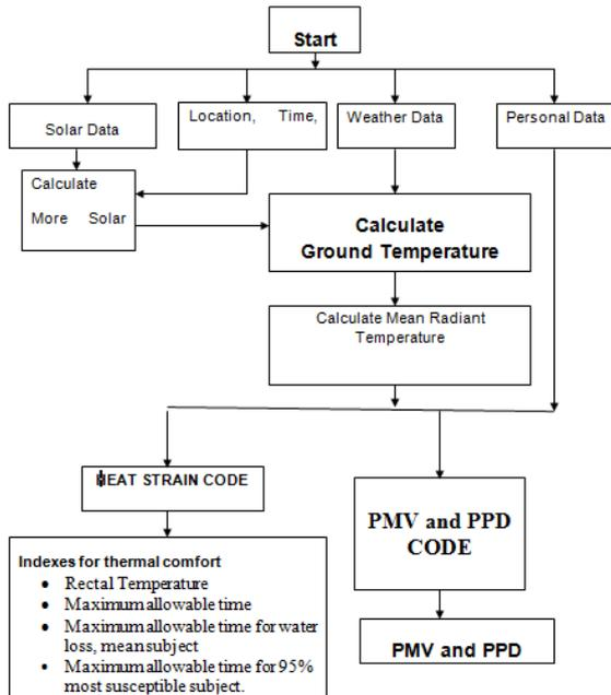
Flow chart showing the general procedure in estimating the thermal comfort indexes.
